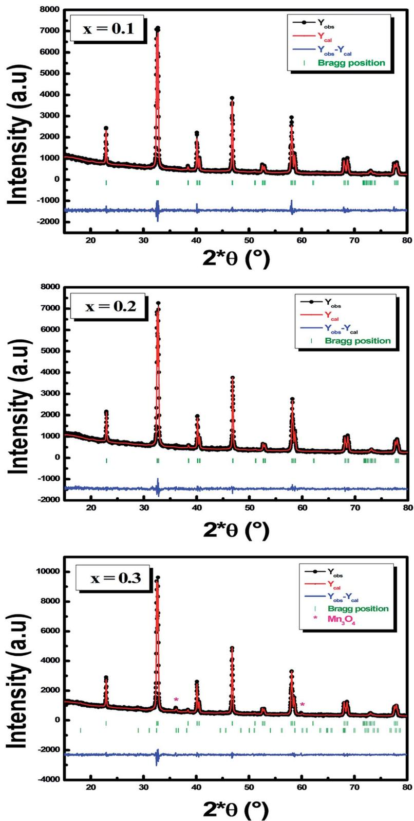
Fig. 2 Rietveld refinement of the X-ray patterns of  $\text{La}_{1-x}\square_x\text{MnO}_3$  ( $x = 0.1, 0.2$  and  $0.3$ ). Experimental data presented in black, calculated data presented in red, difference between them presented in blue, Bragg position presented in green.
