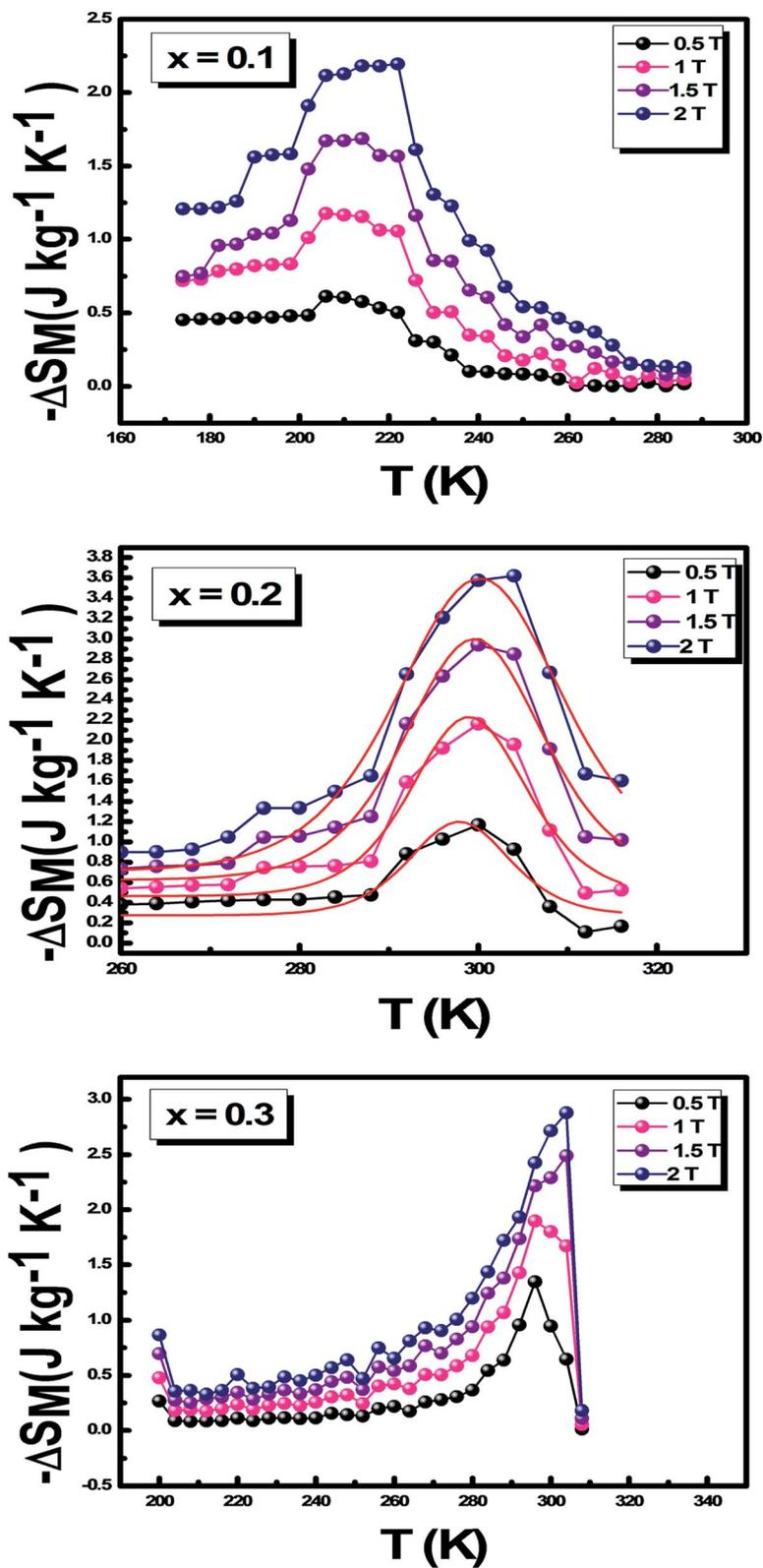
Fig. 7 Thermal variation of the magnetic entropy ( $-\Delta S_M$ ) of  $\text{La}_{1-x}\square_x\text{MnO}_3$  ( $x = 0.1, 0.2$  and  $0.3$ ) systems under different magnetic fields between 0.5 T and 2 T and modeled for  $x = 0.2$ .
