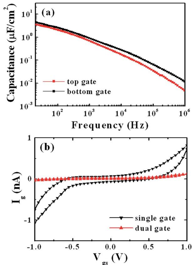
Fig. 2 (a) Specific gate capacitance of the TG and BG dielectrics of such DG TFTs. (b) Leakage current of the STD and DG TFTs.
