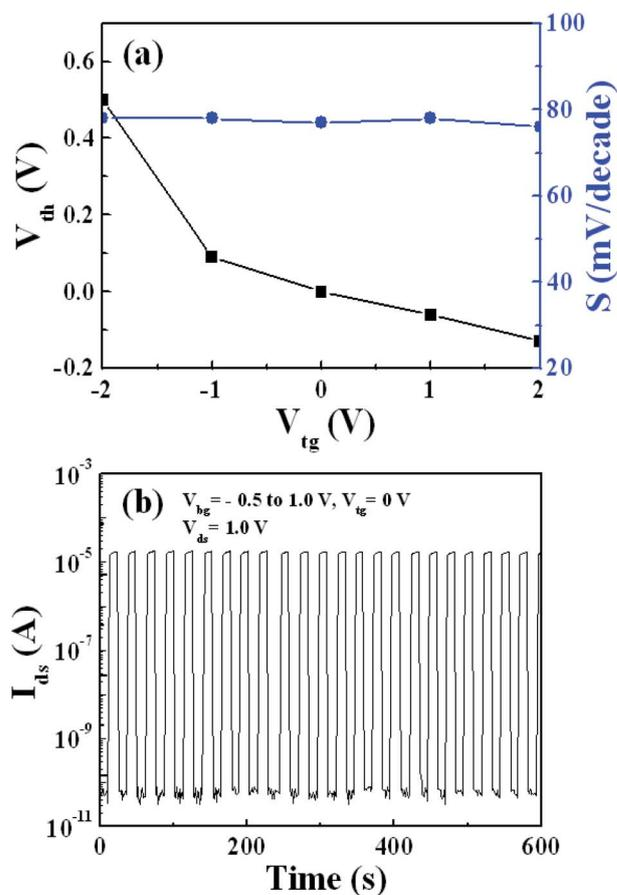
Fig. 5 (a) The threshold voltage and subthreshold swing of the dual gate TFTs at different  $V_{tg}$ . (b) The switching stability driven by square-wave pulses with a period of 1 Hz.
