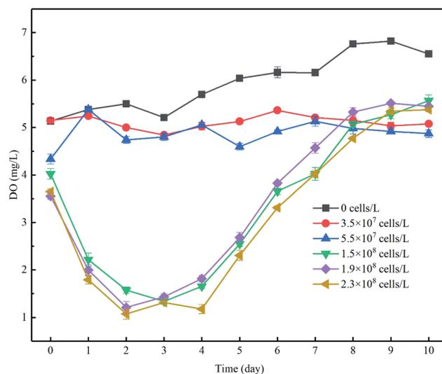
Fig. 3 The changes in DO concentration in the overlying water (mg L<sup>-1</sup>). DO concentrations in each experimental group were assessed, and the most gentle 1 minute DO concentration (calculated the average (C)) data from the real-time DO concentrations are shown. Error bars denote  $\pm 1$  standard error.
