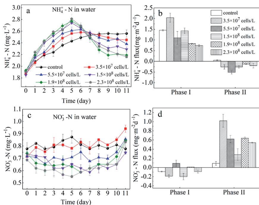
Fig. 4 Sediment to water flux of  $\text{NH}_4^+\text{-N}$  (b) and  $\text{NO}_3^-\text{-N}$  (d) and concentrations of  $\text{NH}_4^+\text{-N}$  (a) and  $\text{NO}_3^-\text{-N}$  (c) in the overlying water. Error bars denote  $\pm 1$  standard error.
