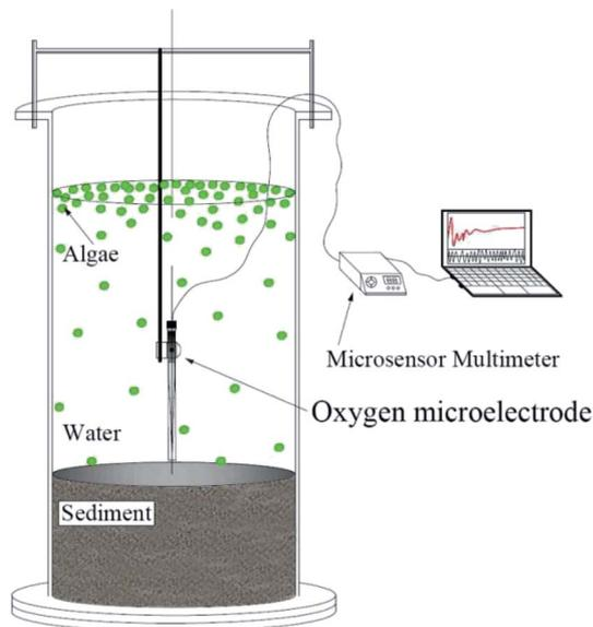
Fig. 1 Schematic diagram of the experimental system.
