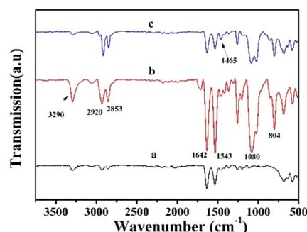
Fig. 4 FTIR spectra of (a) pristine synthetic suede, (b) Synthetic suede-PDMS, and (c) Synthetic suede-PDMS-OTS.
