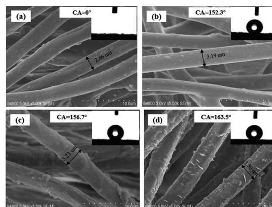
Fig. 2 SEM images of (a) pristine synthetic suede, (b) Synthetic suede–PDMS and (c) Synthetic suede–OTS, (d) Synthetic suede–PDMS–OTS.
