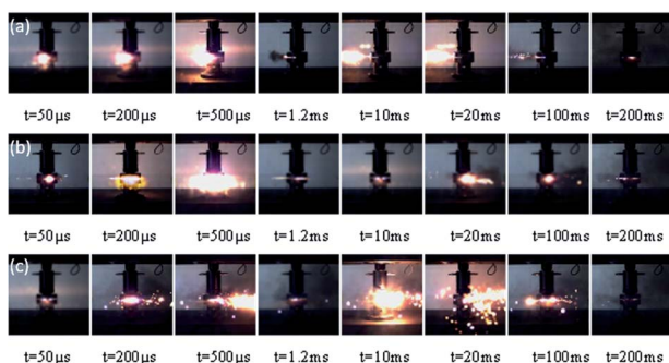
Fig. 9 Reaction phenomena of type A, B and C specimens under quasi-static compression: (a) type A; (b) type B; (c) type C.
