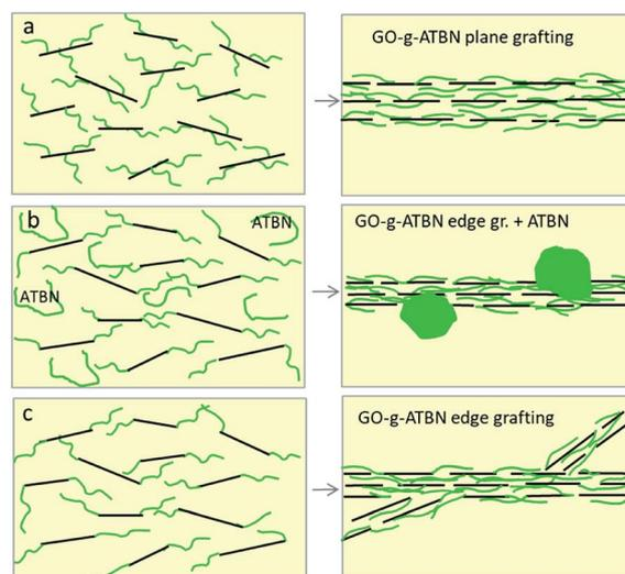
Scheme 2 Effect of grafting geometry on the morphology of lamellar arrays (a) GO-*g*-ATBN<sub>plane</sub> (b) GO-*g*-ATBN<sub>edge</sub> (c) GO-*g*-ATBN<sub>edge</sub> + ATBN.
