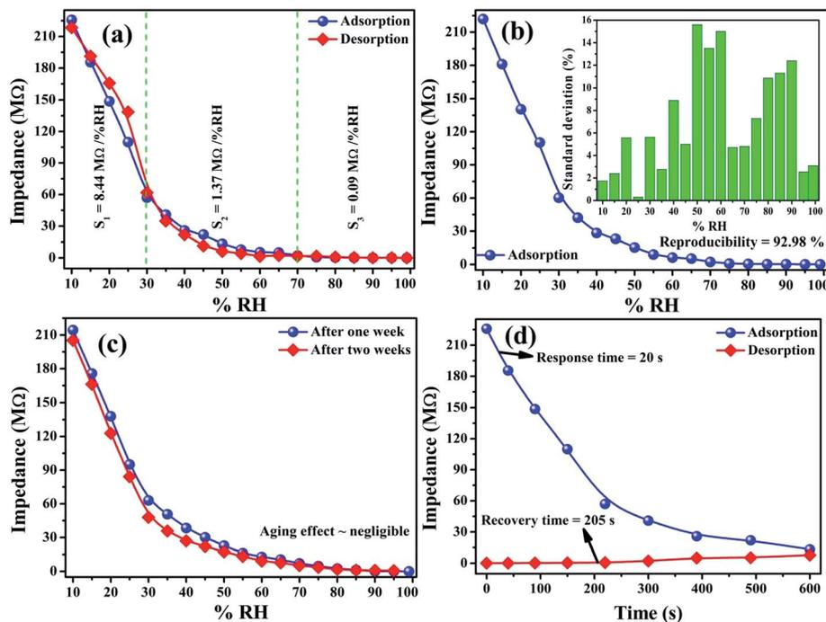
Fig. 3 Sensing performance of the Ru-CuFe<sub>2</sub>O<sub>4</sub> sensor showing (a) sensing response, (b) reproducibility, (c) aging effects and (d) response/recovery time.
