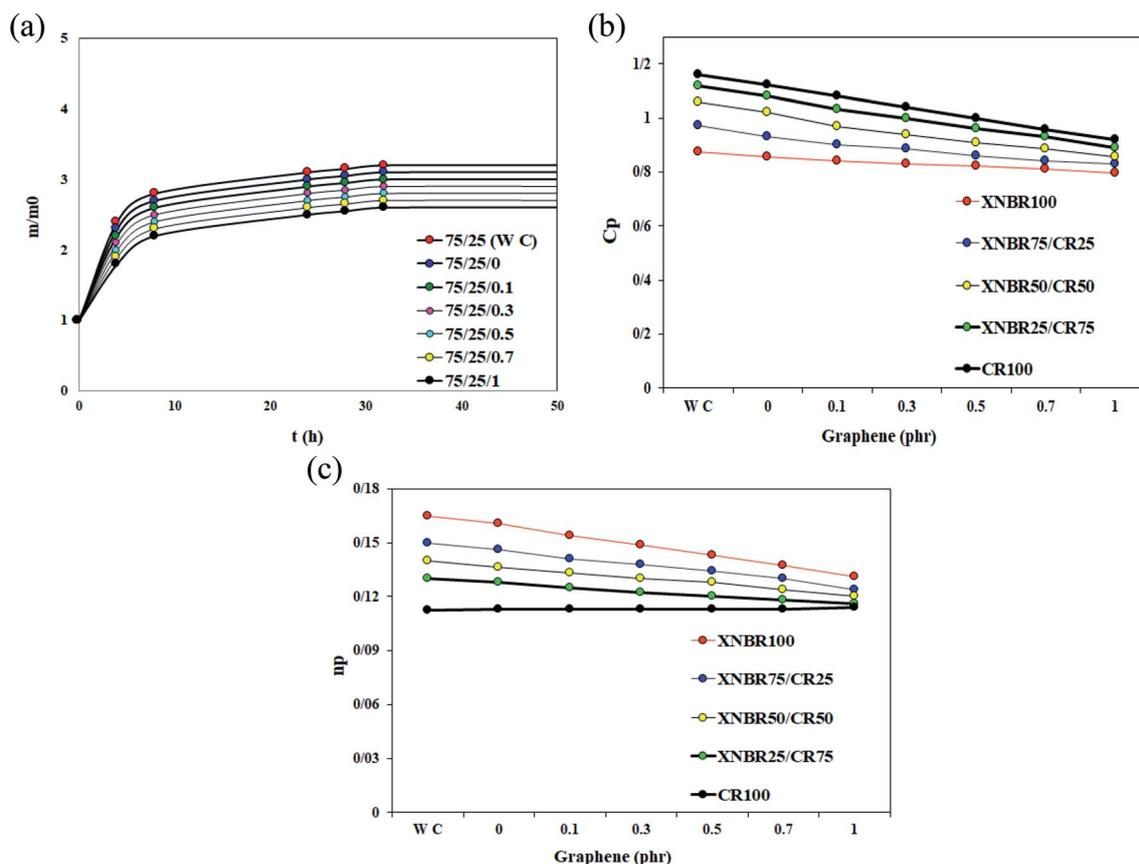
Fig. 3 (a)  $m/m_0$  versus time curves for samples containing the XNBR-*g*-GMA compatibilizer and different amounts of graphene. (b)  $C_p$  versus graphene content for different blends containing the XNBR-*g*-GMA compatibilizer. (c)  $n_p$  versus graphene content for different blends containing the XNBR-*g*-GMA compatibilizer.
