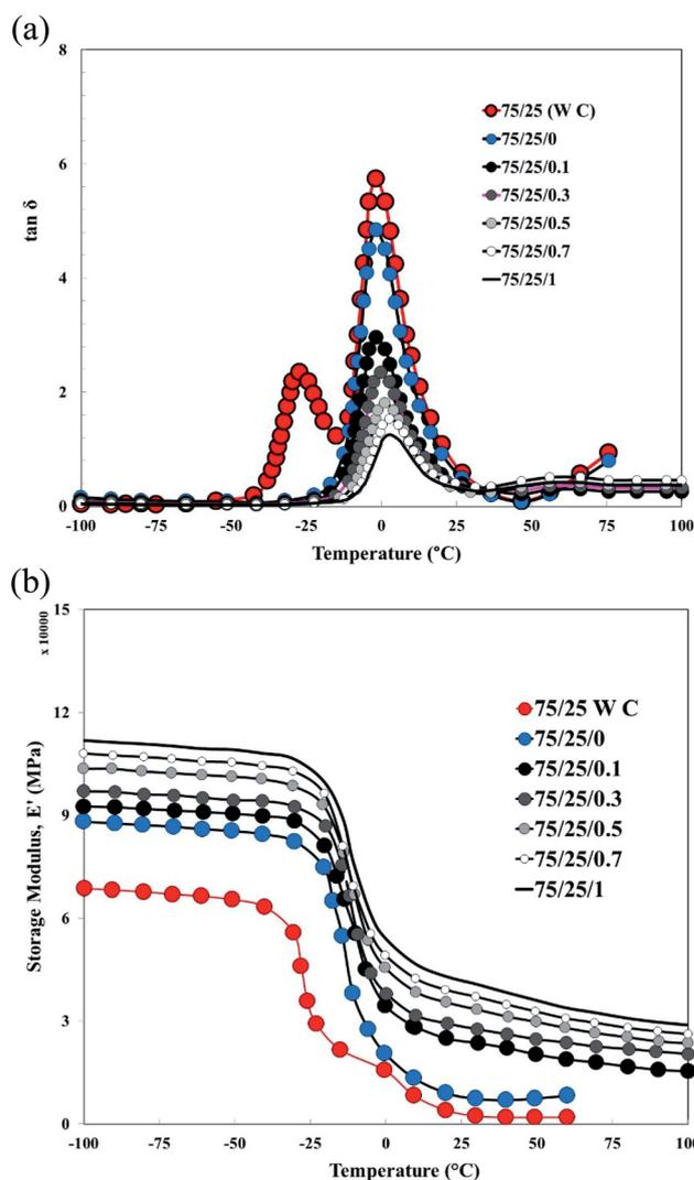
Fig. 8 (a) Loss factor versus temperature curves of XNBR75/CR25 nanocomposites (effect of graphene and compatibilizer). (b) Storage modulus ( $E'$ ) versus temperature curves of XNBR75/CR25 nanocomposites (effect of graphene and compatibilizer).
