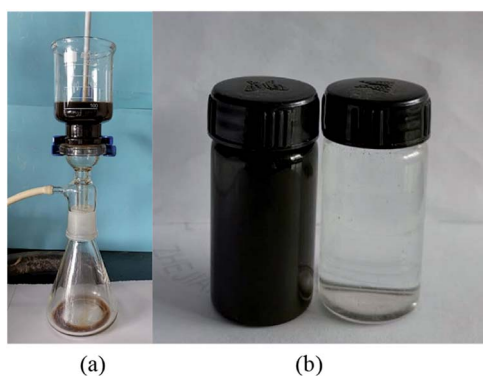
Fig. 9 Separation of asphalt-containing oil–water mixtures with PDCCP aerogel: (a) experimental setup; (b) filtrate phase (left) and residual phase (right).
