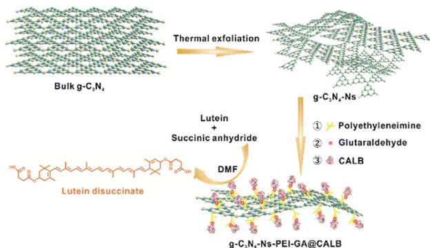
Scheme 1 Schematic representation of the formation of g-C 3 N 4 -Ns-PEI-GA@CALB.
