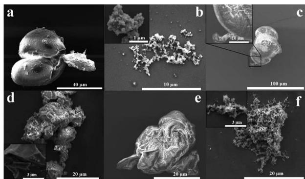
Fig. 4 SEM images of PSF for (a) commercial material, (b) material formed using conventional batch processing, (c) material formed in the VFD at the optimised conditions ( $T_{22}$  at 6000 rpm, 160 °C, 45°, and 60 min). PSF characterized in the VFD at 6000 rpm, 160 °C,  $\theta$  45° for (d) 15 min, (e) 30 min, and (f) 90 min reaction time. All the sample were drop cast and coated with ca. 5 nm layer of Pt.
