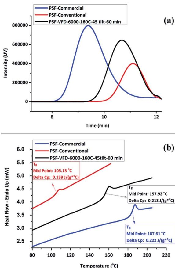
Fig. 3 Comparison between (a) GPC traces (UV detector) and (b) DSC thermograms of commercial, conventional and VFD synthesized PSF ( $T_{22}$  at 6000 rpm, 160 °C, 45°, and 60 min). (b) Temperature scan in  $T_g$  measurements were conducted between 30 °C and 230 °C at 10 °C min<sup>-1</sup>.
