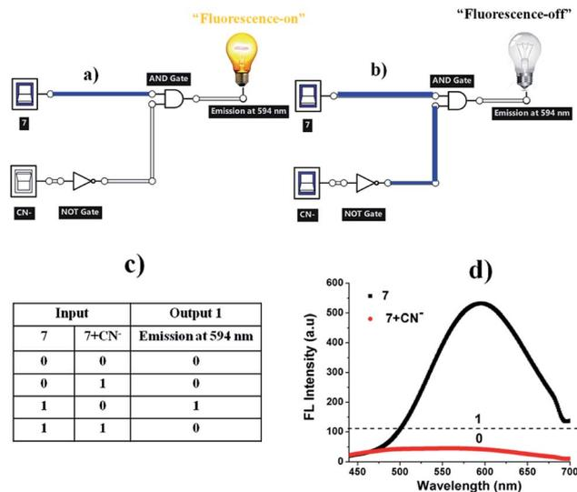
Fig. 12 (a) "Fluorescence-on" and (b) "fluorescence-off" logic circuit for 7 and 7 + CN<sup>-</sup>. (c) Corresponding truth table and (d) fluorescence spectra of 7 in the presence of CN<sup>-</sup> (12 equiv.).
