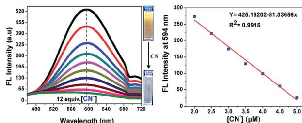
Fig. 4 Fluorescence spectra changes of probe 7 in acetonitrile upon the addition of different concentrations of aqueous CN<sup>-</sup> anion upon excitation at 370 nm (left) and a linear calibration curve of the emission band intensity at 594 nm *versus* concentration of CN<sup>-</sup> in the range of 2 to 5 μM (right).
