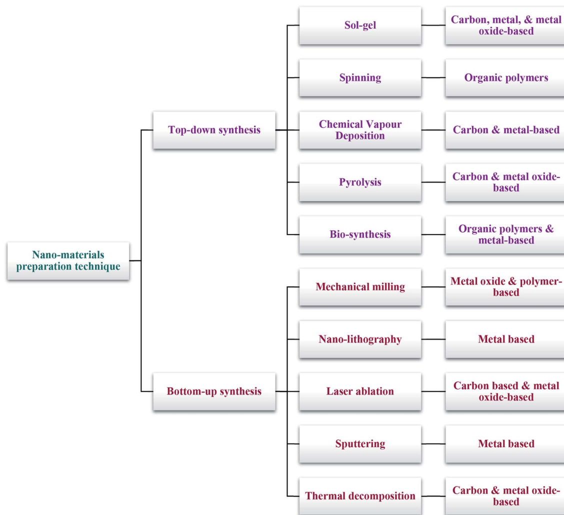
Scheme 2 Conventional synthetic techniques for nano-materials.
