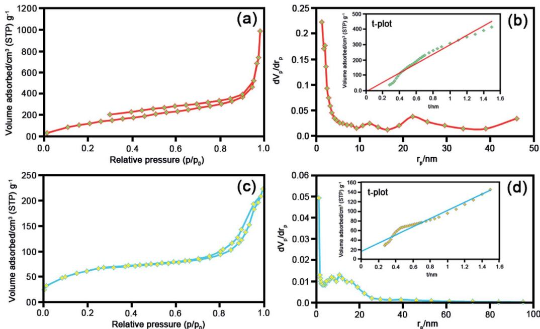
Fig. 7 BET analyses, BJH and *t* plots of the as-synthesized (a) and (b) raw Y zeolite, (c) and (d) CoFe<sub>2</sub>O<sub>4</sub>@Cr-MIL-101/Y.
