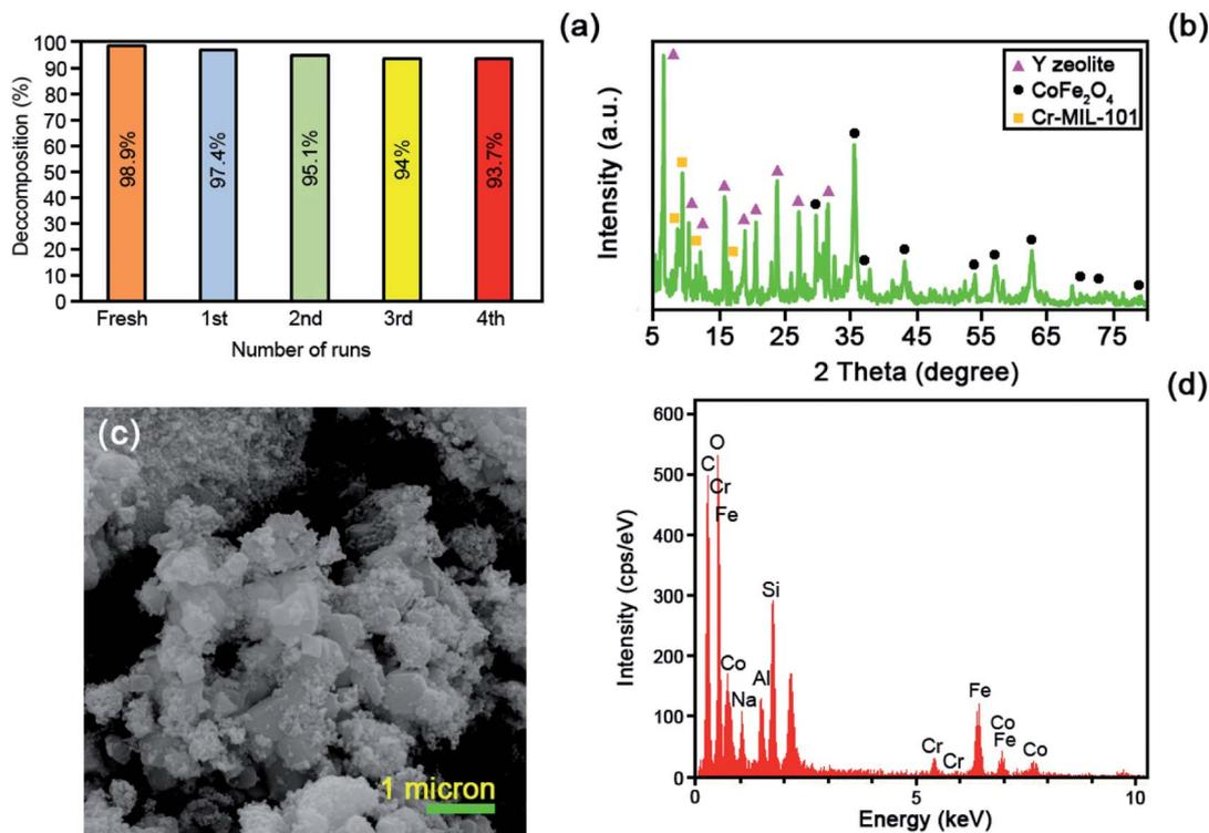
Fig. 10 (a) The regeneration plot, (b) XRD (c) FESEM, and (d) EDS analyses of the recovered CoFe<sub>2</sub>O<sub>4</sub>/Y@Cr-MIL-101 on the sonodecomposition process of MB after four runs (optimized experimental conditions; irradiation time: 60 min, [MB]<sub>0</sub>: 25 mg L<sup>-1</sup> (50 mL), [H<sub>2</sub>O<sub>2</sub>]: 40 mmol L<sup>-1</sup> (2 mL), [catalyst dosage]: 0.5 g L<sup>-1</sup>, pH: 7 and temperature: 25 ± 1 °C).
