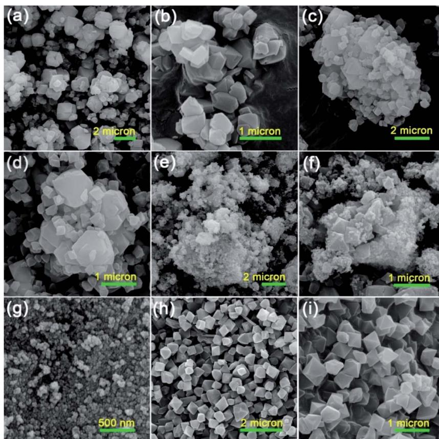
Fig. 3 FESEM images of the as-synthesized (a and b) raw Y zeolite, (c and d) Cr-MIL-101/Y, (e and f)  $\text{CoFe}_2\text{O}_4$ @Cr-MIL-101/Y, (g) raw  $\text{CoFe}_2\text{O}_4$ , (h and i) raw Cr-MIL-101 with different resolutions.
