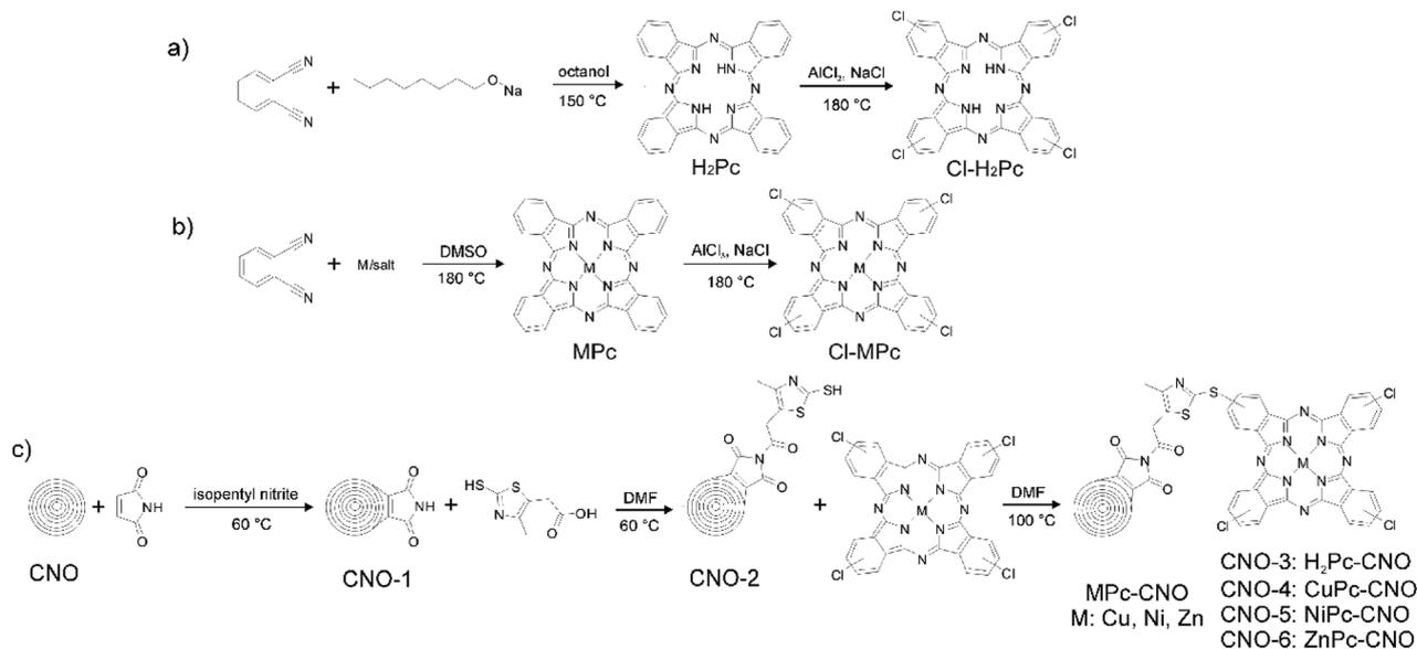
Fig. 1 Schematic illustration of the whole synthesis procedure for (a) Pc, (b) MPc, and (c) Pc-CNO and MPc-CNO derivatives.
