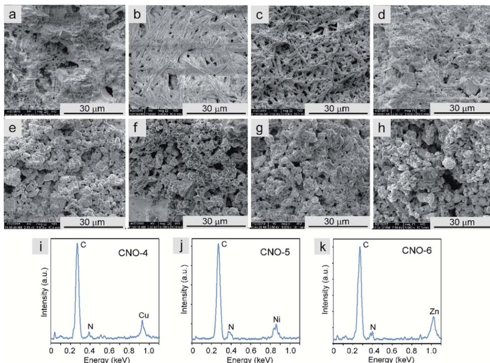
Fig. 5 (a–h) SEM images of (a) H<sub>2</sub>Pc, (b) CuPc, (c) NiPc, (d) ZnPc, (e) CNO-3, (f) CNO-4, (g) CNO-5 and (h) CNO-6. (i–k) Energy dispersive X-ray spectroscopy analyses of (i) CNO-4, (j) CNO-5 and (k) CNO-6.
