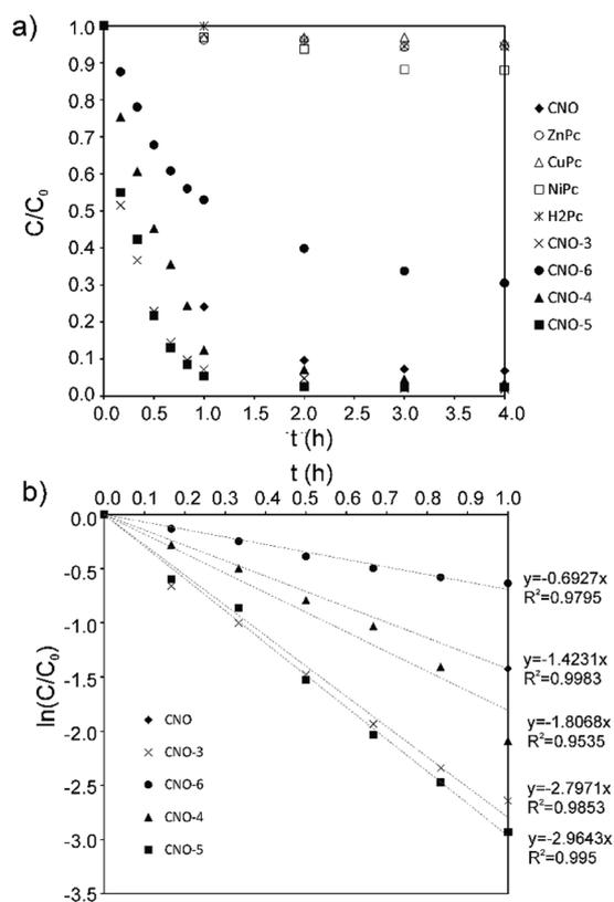
Fig. 7 (a) The photocatalytic degradation profiles obtained for RhB with CNO, H<sub>2</sub>Pc, MPCs and MPC-CNOs. (b) The photocatalytic RhB degradation kinetics obtained with CNO and MPC-CNOs.
