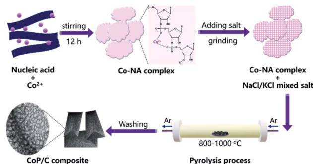
Fig. 1 Schematic illustration of the synthesis procedure of a cobalt phosphide/carbon composite.
