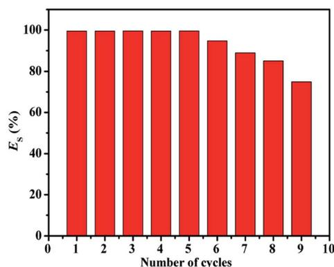
**Fig. 7** Efficiency of Fe<sub>3</sub>O<sub>4</sub>@HA@PDDA MNPs for separating an oil–water emulsion at each of a nine-cycle sequence.
