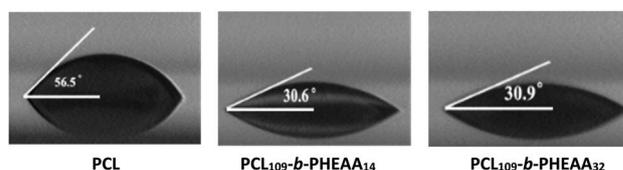
Fig. 3 Contact angle of PCL and copolymer.
