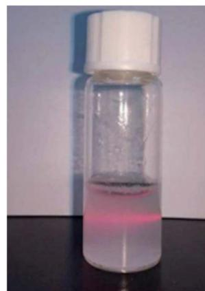
Fig. 2 Tyndall effect of PCL-*b*-PHEAA.
