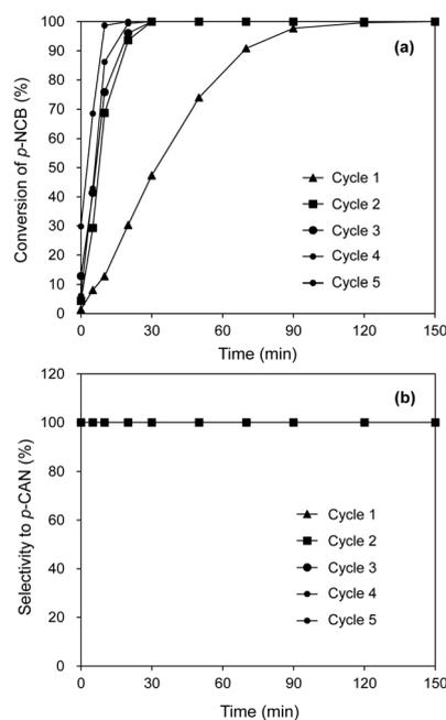
Fig. 7 The reuse of Pt/Al<sub>2</sub>O<sub>3</sub>@NC-25 for catalytic hydrogenation of *p*-CNB. Reaction conditions: catalyst dosage: 20 mg, alcohol: 20 ml, *p*-CNB amount: 100 mg, reaction temperature: 80 °C, H<sub>2</sub> pressure: 1 MPa.
