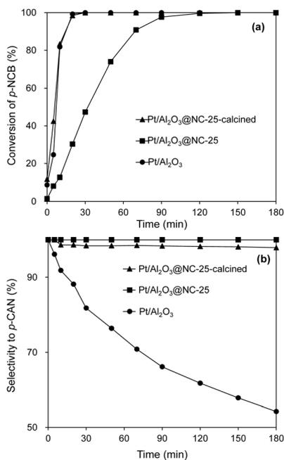
Fig. 6 Catalytic hydrogenation of *p*-CNB on Pt/Al<sub>2</sub>O<sub>3</sub>@NC-25-calcined in comparison with Pt/Al<sub>2</sub>O<sub>3</sub>@NC-25 and Pt/Al<sub>2</sub>O<sub>3</sub>. Reaction conditions: catalyst dosage: 20 mg, alcohol: 20 ml, *p*-CNB amount: 100 mg, reaction temperature: 80 °C, H<sub>2</sub> pressure: 1 MPa.
