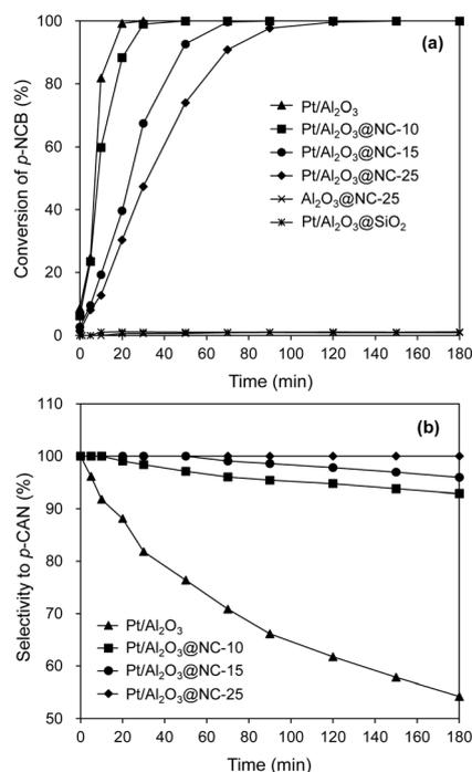
Fig. 5 Catalytic hydrogenation of *p*-CNB on the catalysts. Reaction conditions: catalyst dosage: 20 mg, alcohol: 20 ml, *p*-CNB amount: 100 mg, reaction temperature: 80 °C, H<sub>2</sub> pressure: 1 MPa.
