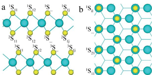
Fig. 1 The (a) side and (b) top views of the 2-layered 3R MoS<sub>2</sub> (the number of superscripts represents the layer of S atoms, and the first and second subscripts represent the row and column of S atoms, respectively).
