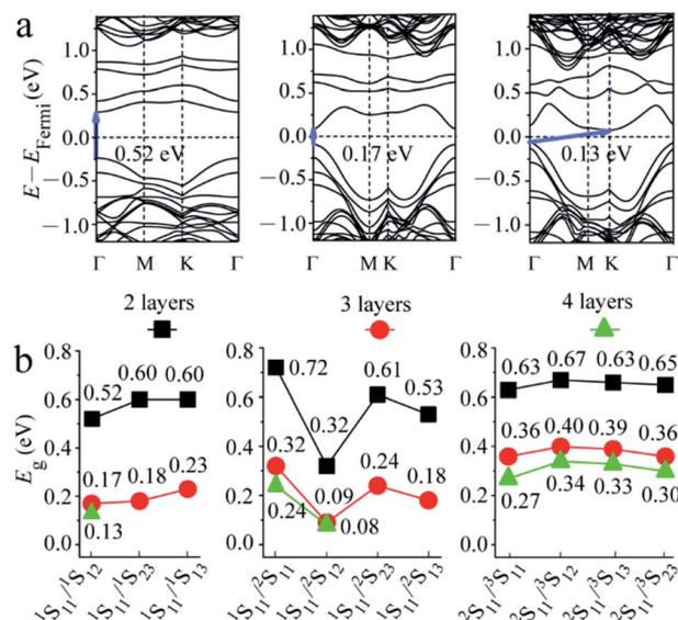
Fig. 3 (a) Band structures for 2-, 3-, and 4-layered MoS<sub>2</sub> with <sup>1</sup>S<sub>11</sub>/<sup>1</sup>S<sub>12</sub> combinational vacancies as an example and (b) the gaps of the intermediate band in the band gap ( $E_g$ ) for 2-, 3-, and 4-layered MoS<sub>2</sub> with two S vacancies at 4% bulk concentrations.
