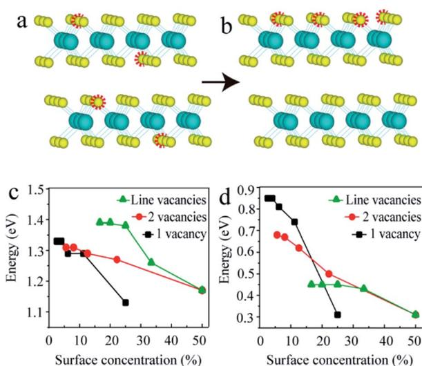
Fig. 4 (a) Schematic diagram of vacancies on average. (b) Schematic diagram of vacancies on the top S layer. (c) The gaps of intrinsic and (d) intermediate bands in the band gaps for  $n \times n$  ( $n = 2, 3, \dots, 6$ ) supercells with one (black) and two (red) adjacent point vacancies and line (green) vacancies.
