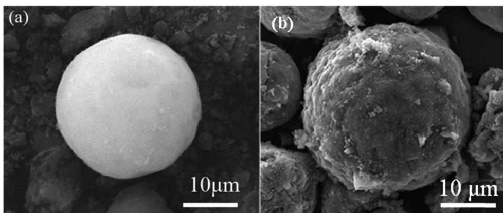
Fig. 4 SEM images of (a) SiO<sub>2</sub>·2H<sub>2</sub>O and (b) PPQA@SiO<sub>2</sub>.
