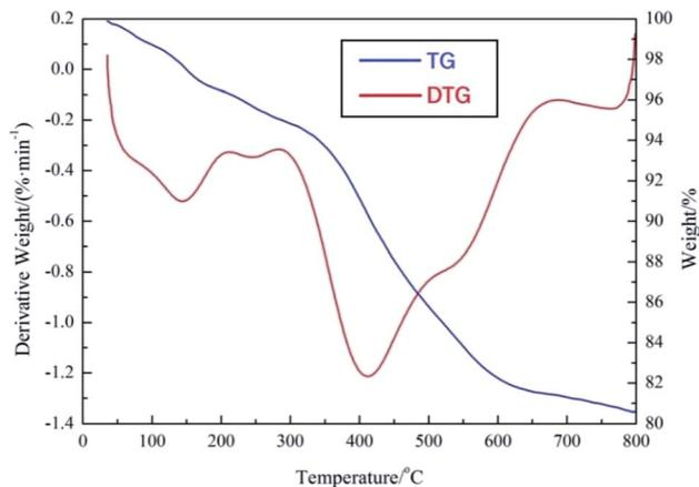
Fig. 5 TG/DTG analysis of demulsifier PPQA@SiO<sub>2</sub>.
