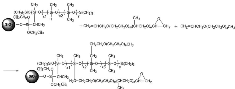
(c) Synthesis of PSS@SiO<sub>2</sub>
