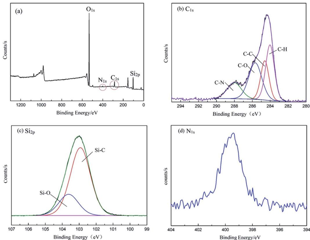
Fig. 3 (a) XPS spectra of PPQA@SiO<sub>2</sub>, (b) high-resolution C1s spectrum, (c) high-resolution Si2p spectrum, and (d) high-resolution N1s spectrum.
