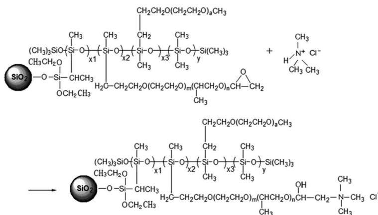
(d) Synthesis of PPQA@SiO<sub>2</sub>Fig. 1 Synthesis steps of supported demulsifier PPQA@SiO<sub>2</sub>.
