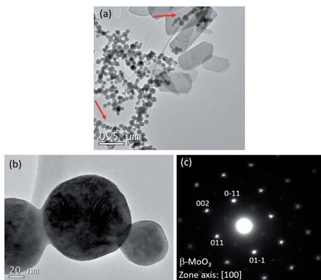
Fig. 5 TEM images of MoO<sub>3</sub> nanostructures grown on the plate electrodes. (a) Several nanoplates and arrangements of nanospheres (b) nanospheres. (c) Diffraction pattern of a region with nanospheres corresponding to  $\beta$ -MoO<sub>3</sub> phase.
