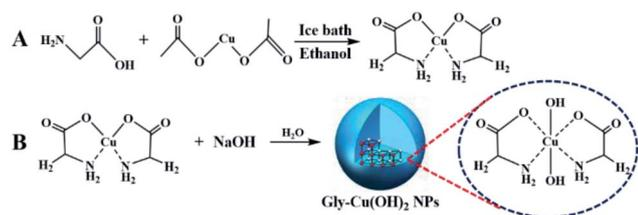
Fig. 1 Schematic preparation of Gly-Cu(OH)<sub>2</sub> NPs.
