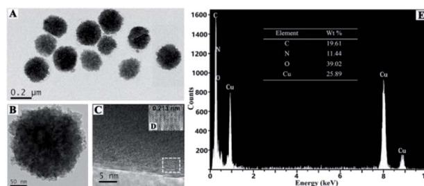
Fig. 2 TEM images of Gly-Cu(OH)<sub>2</sub> NPs synthesized from Cu(Gly)<sub>2</sub> (A and B). HRTEM image of (C) the edge of Gly-Cu(OH)<sub>2</sub> nanoparticle and (D) some individual Cu(OH)<sub>2</sub> NPs (crystallites). EDS pattern of Gly-Cu(OH)<sub>2</sub> NPs (E).
