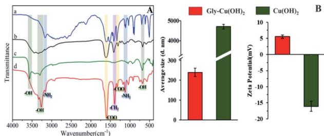
Fig. 3 (A) FTIR spectra of (a) glycine, (b) *cis*-Cu(Gly)<sub>2</sub>, (c) Cu(OH)<sub>2</sub>, (d) Gly-Cu(OH)<sub>2</sub>. (B) Particle average size and zeta potential of Cu(OH)<sub>2</sub> microparticles and Gly-Cu(OH)<sub>2</sub> NPs. The bars in the figure represent standard deviation ( $\pm$ SD).
