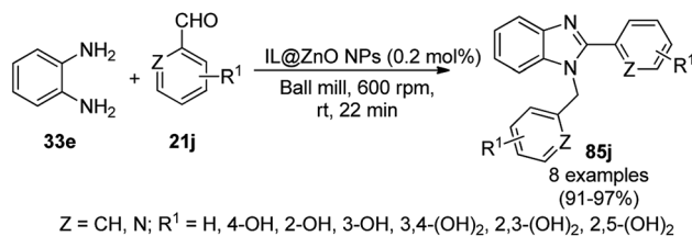
Scheme 193 IL@ZnO NP-catalyzed synthesis of 1,2-disubstituted benzimidazoles ( 85j ) reported by Singh et al.
