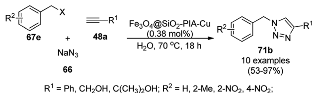
Scheme 266 Synthesis of triazole via the click reaction among alkyl halides (67e), alkynes (48a) and 66 in the presence of a catalyst such as Cu(II) complex on Fe 3 O 4 @SiO 2 NPs. 479
