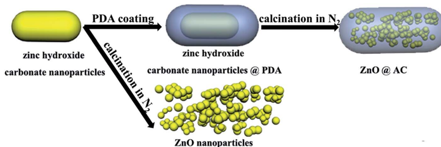
Fig. 1 Schematic of the fabrication process of ZnO@AC and pure ZnO NPs.
