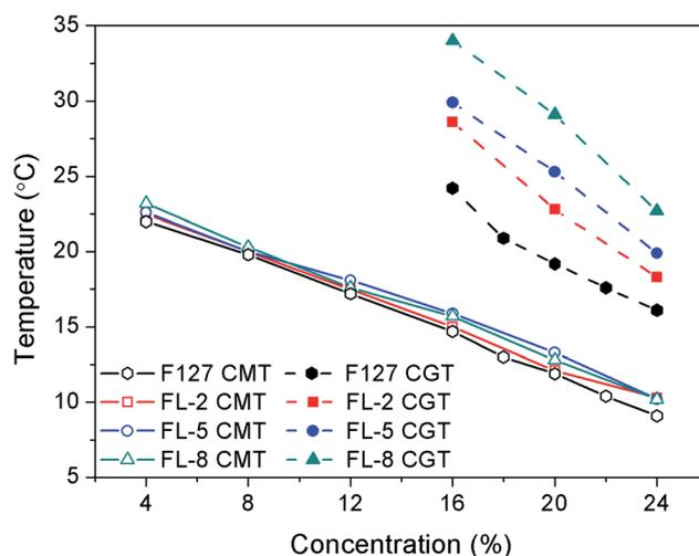
Fig. 3 CMT and CGT of F127 and FL hydrogels measured by differential scanning calorimeter.
