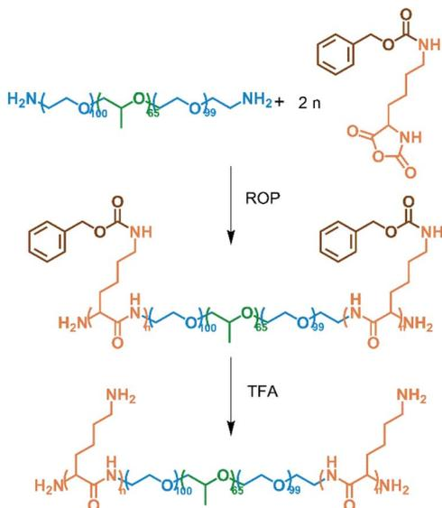
**Scheme 1** Synthetic route of FL polymer. The amino-terminated F127 initiates the ring-opening polymerization of *L*-lysine(z)-NCA and the deprotection reaction in the environment of trifluoroacetic acid.
