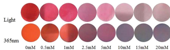
Fig. 5 Hcy-Mo (1 mM) with different concentrations of sodium bisulfite (0, 0.5, 1, 2.5, 5, 10, 15, and 20 mM) in sunlight and 365 nm fluorescent light.
