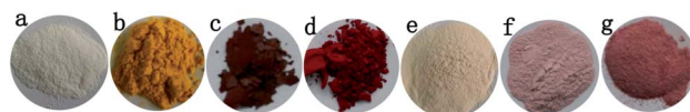
Fig. 5 Photo images of \text{TiO}_2 (a), PDI-1 (b), PDI-2 (c), PDI-3 (d), PDI-1/TiO 2 (e), PDI-2/TiO 2 (f) and PDI-3/TiO 2 (g).
