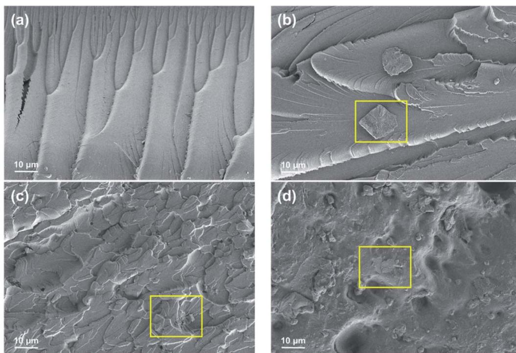
Fig. 12 Micrograph images of the fracture surface after tensile testing (a) photo-curable PU, (b) PU-graphene (PU-G), (c) PU-0.6% lignin/G, and (d) top surface of PU-0.6% lignin/G. Reprinted with permission from ref. 95. Copyright 2019 *Polymers*.
