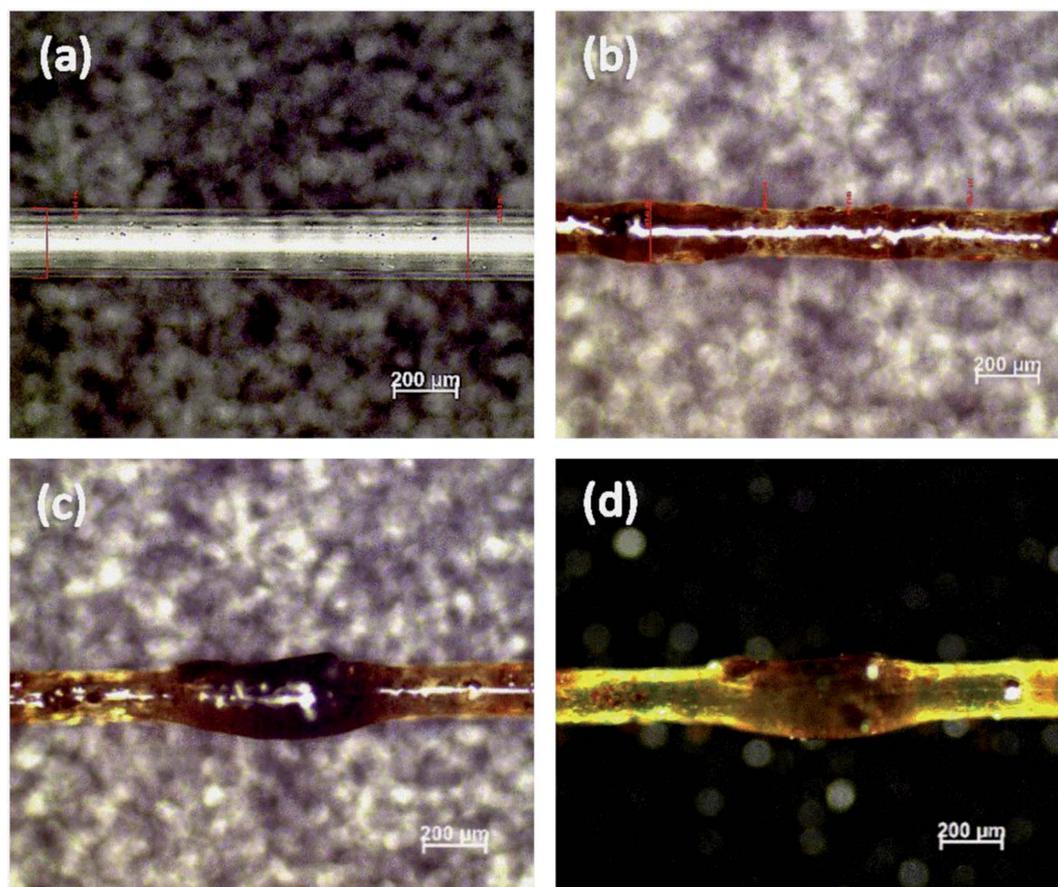
Fig. 13 Light micrographs of (a) individual PLA fibers extruded from 0.2 mm nozzle 20 mm s<sup>-1</sup> printing speed; (b) individual PLA blends with 5 wt% lignin fibers extruded from 0.2 mm nozzle 20 mm s<sup>-1</sup> printing speed; (c and d) individual PLA blends with 5 wt% lignin fibers extruded from 0.2 mm nozzle 60 mm s<sup>-1</sup> printing speed. Reprinted with permission from ref. 140. Copyright 2017 *Manufacturing Review*.
