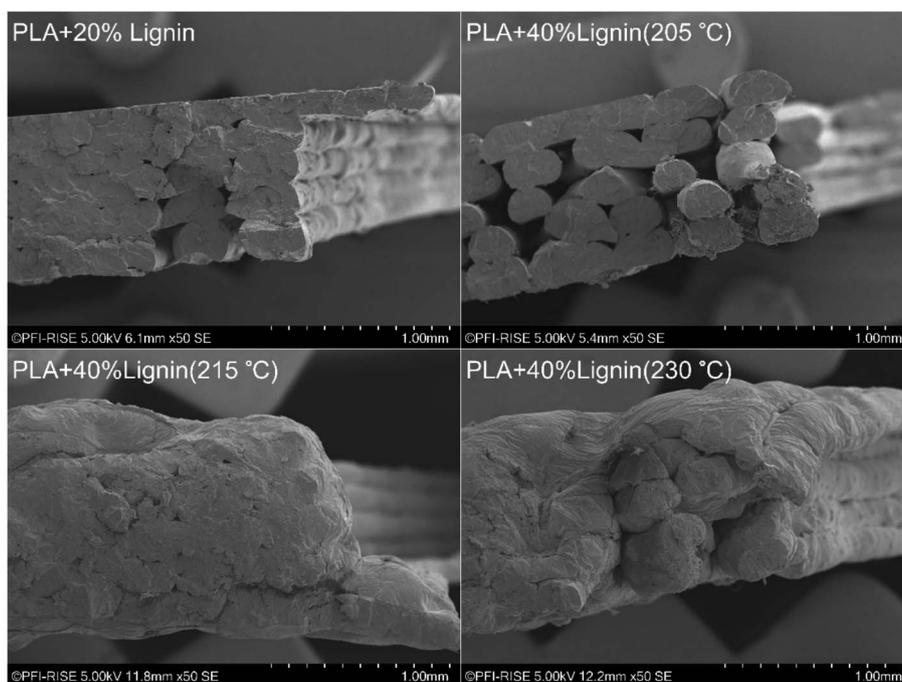
Fig. 11 Scanning electron microscopy (SEM) analysis of the fracture surface of tensile tested dogbones. Reprinted with permission from ref. 87. Copyright 2019 *Materials*.
