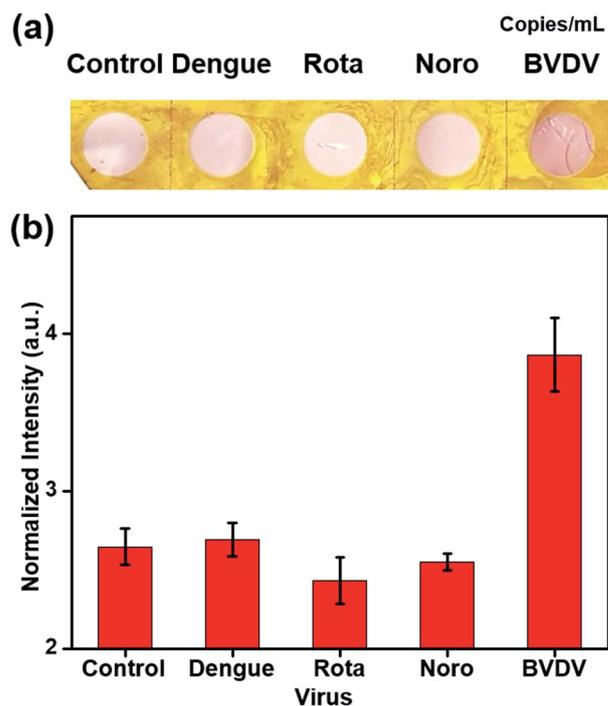
Fig. 4 Selectivity evaluation of the intensity of BVDV peptide #2 with different types of viruses, dengue virus type II, rotavirus, norovirus ( $10^5$  copies per mL) as negative controls to confirm the capture affinity of peptides. (a) Smartphone camera images for dot-blot assay of different types of viruses by using AuNPs@BVDV peptide #2. (b) Normalized intensity of UV-vis reflection spectrum for quantification ( $n = 3$ ).
