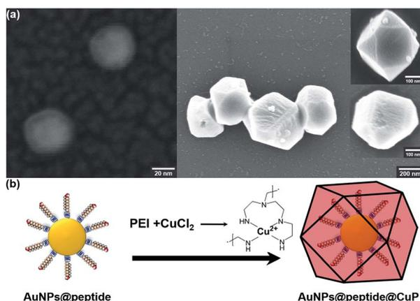
**Fig. 1** Formation of AuNPs and AuNPs@copper nano-polyhedral shell. (a) Structural analysis of the AuNPs (left) and AuNPs@CuP nanostructure (right; scale bar: 200 nm) based on SEM (inset: the cuboctahedrons and five-fold rods; scale bars: 100 nm). (b) Schematic representation of Cu and polyethyleneimine (PEI)-covered growth of CuP nanostructure by highly specific CuP growth on the AuNPs.
