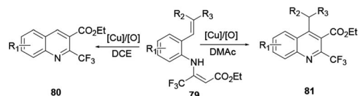
Scheme 21 Synthesis of 2-trifluoromethylquinoline.
