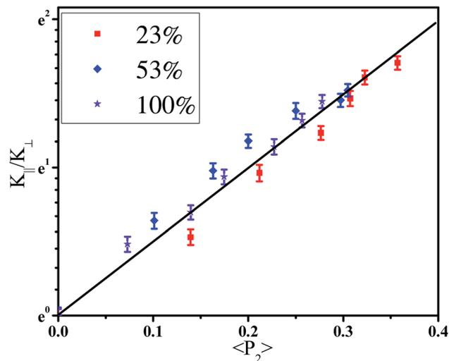
Fig. 8 Change of the logarithm of anisotropy of thermal conductivity  $K_{\parallel}/K_{\perp}$  with the orientation degree  $\langle P_2 \rangle$  of backbone bonds for different composition ratio of styrene. ( $T = 300$  K,  $\alpha = 50$  nm ns $^{-1}$ .)
