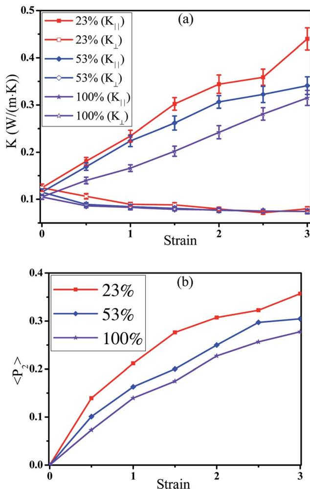
Fig. 7 Change of the thermal conductivities (a)  $K_{\parallel}$  (W m $^{-1}$  K $^{-1}$ ) parallel to tensile direction,  $K_{\perp}$  (W m $^{-1}$  K $^{-1}$ ) perpendicular to tensile direction, and (b) the orientation degree  $\langle P_2 \rangle$  of backbone bonds with the strain for different composition ratio of styrene. ( $T = 300$  K,  $\alpha = 50$  nm ns $^{-1}$ .)
