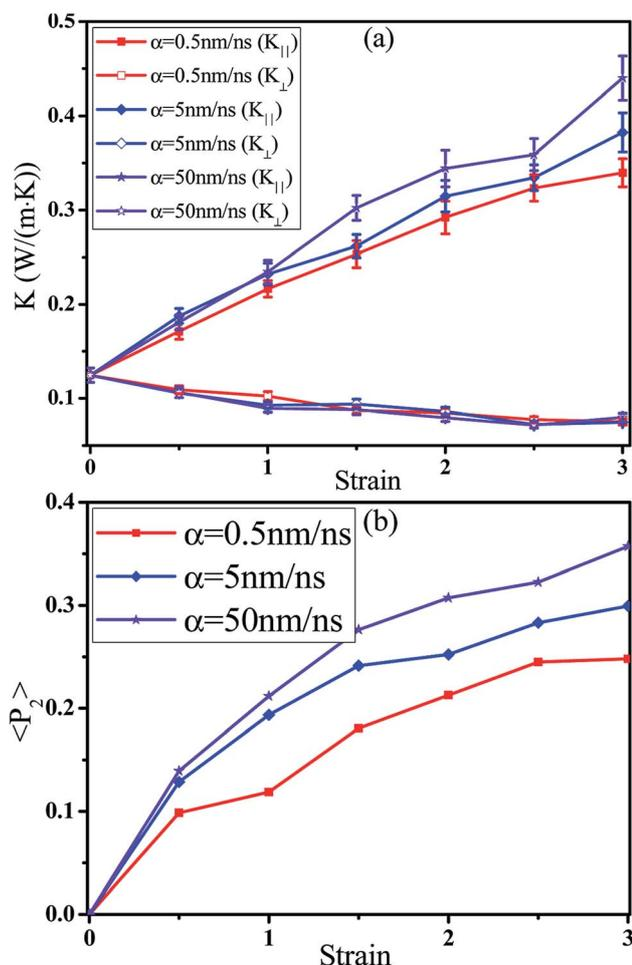
Fig. 5 Change of the thermal conductivities (a)  $K_{\parallel}$  ( $\text{W m}^{-1} \text{ K}^{-1}$ ) parallel to tensile direction,  $K_{\perp}$  ( $\text{W m}^{-1} \text{ K}^{-1}$ ) perpendicular to tensile direction, and (b) the orientation degree  $\langle P_2 \rangle$  of backbone bonds with the strain for different tensile rates  $\alpha$ . ( $T = 300 \text{ K}$ , composition ratio of styrene = 23%.)
