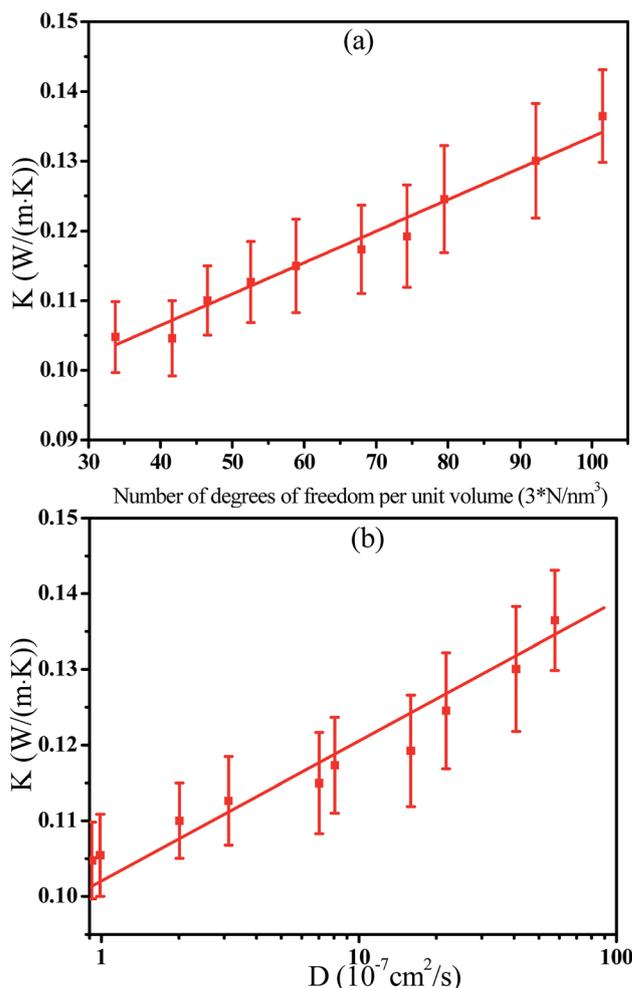
Fig. 4 The thermal conductivity  $K$  of the butadiene styrene rubber as a function of (a) the degrees of freedom of backbone atoms per unit volume and (b) the logarithm of diffusion coefficient ( $D$ ) of backbone atoms. ( $T = 300 \text{ K}$ , strain = 0.0.)
