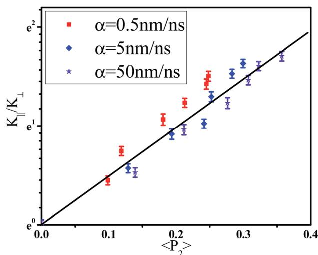
Fig. 6 Change of the logarithm of anisotropy of thermal conductivity  $K_{\parallel}/K_{\perp}$  with the orientation degree  $\langle P_2 \rangle$  of backbone bonds for different tensile rates  $\alpha$ . ( $T = 300 \text{ K}$ , composition ratio of styrene = 23%.)
