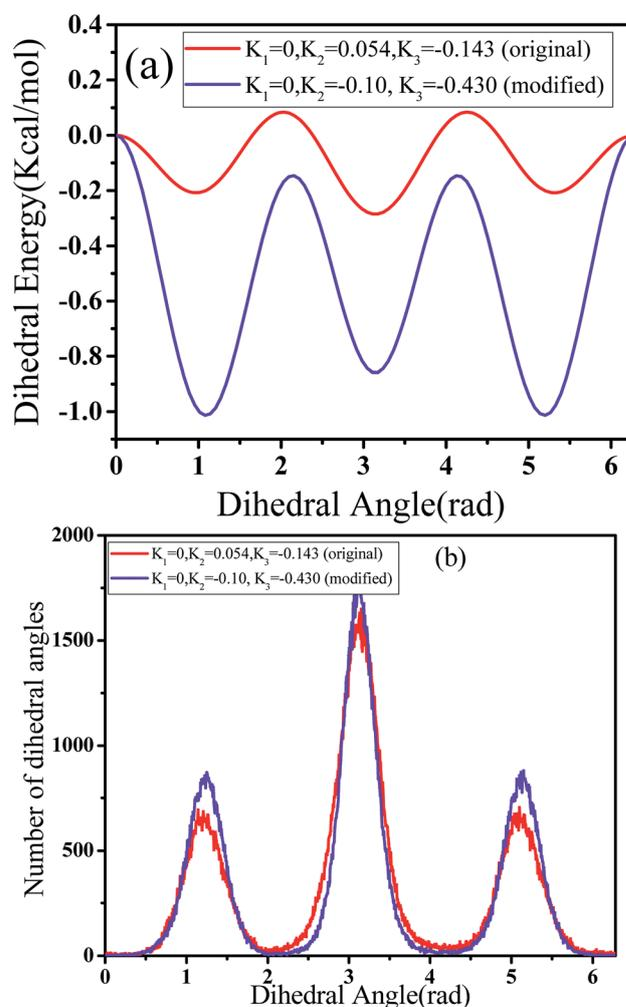
Fig. 10 (a) Dihedral energy and (b) number of dihedral angles for the original and modified dihedral parameters at strain = 3.0. ( $T = 300$  K, composition ratio of styrene = 23%,  $\alpha = 50$  nm ns<sup>-1</sup>.)
