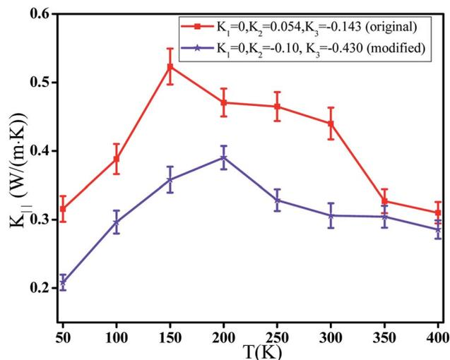
Fig. 11 Change of the thermal conductivities  $K_{\parallel}$  ( $W m^{-1} K^{-1}$ ) parallel to tensile direction with the temperature ( $T$ ) for the original and modified dihedral parameters at strain = 3.0. (Composition ratio of styrene = 23%,  $\alpha = 50 \text{ nm ns}^{-1}$ .)
