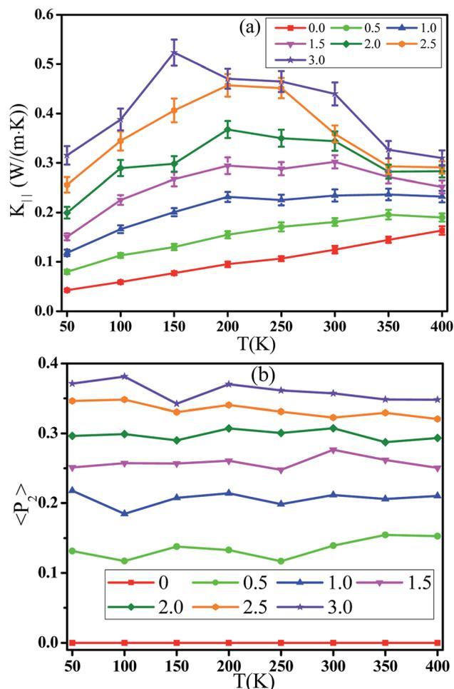
Fig. 9 Change of the (a) thermal conductivities  $K_{\parallel}$  (W m $^{-1}$  K $^{-1}$ ) parallel to tensile direction and (b) the orientation degree  $\langle P_2 \rangle$  of backbone bonds with the temperature ( $T$ ) for different strains. (Composition ratio of styrene = 23%,  $\alpha = 50$  nm ns $^{-1}$ .)
