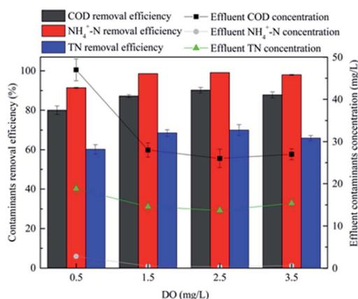
Fig. 4 Effluent concentration and removal efficiency of COD and nitrogen in A<sup>2</sup>/O-MABR system at various DO.
