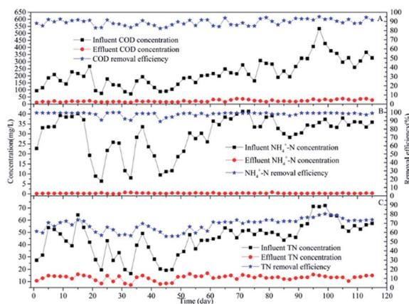
Fig. 5 Concentration of influent and effluent and removal efficiency in A<sup>2</sup>/O-MABR system at optimal operation parameters: (A) COD; (B) NH<sub>4</sub><sup>+</sup>-N; (C) TN.
