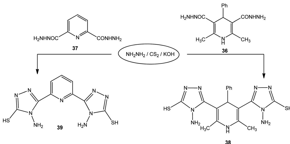
Scheme 13 Synthesis of bis-triazoles 38 and 39.
