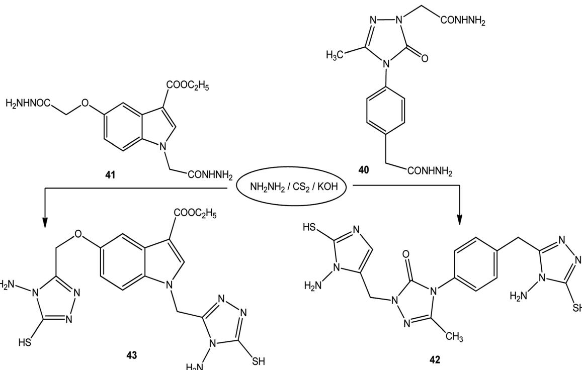
Scheme 14 Synthesis of bis-triazoles 42 and 43.
