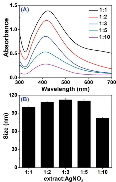
Fig. 3 (A) UV-Vis spectra of the mixtures after 1 h reaction between *Cornus officinalis* extract and AgNO<sub>3</sub> under 365 nm UV radiation at different proportions; (B) the size of AgNPs obtaining at (A).
