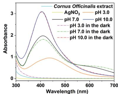
Fig. 1 UV-Vis spectra of the mixture after 1 h reaction between *Cornus officinalis* extract and AgNO<sub>3</sub> with/without 365 nm UV radiation at different pH.
