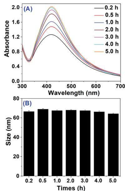
Fig. 4 (A) UV-Vis spectra of the mixture after the reaction between *Cornus officinalis* aqueous extract and AgNO<sub>3</sub> under 365 nm UV radiation at different times; (B) the size of AgNPs obtaining at (A).
