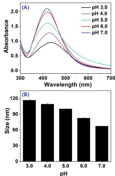
Fig. 2 (A) UV-Vis spectra of the mixture after 1 h reaction between *Cornus officinalis* extract and AgNO<sub>3</sub> under 365 nm UV radiation at different pH; (B) the size of AgNPs obtaining at (A).
