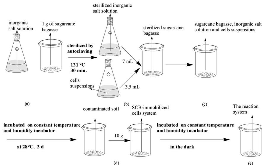
Scheme 2 The reaction system set-up.
