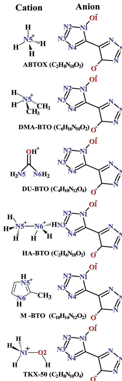
Fig. 1 Chemical structures of 5,5'-bitetrazole-1,1'-diolate based energetic salts.
