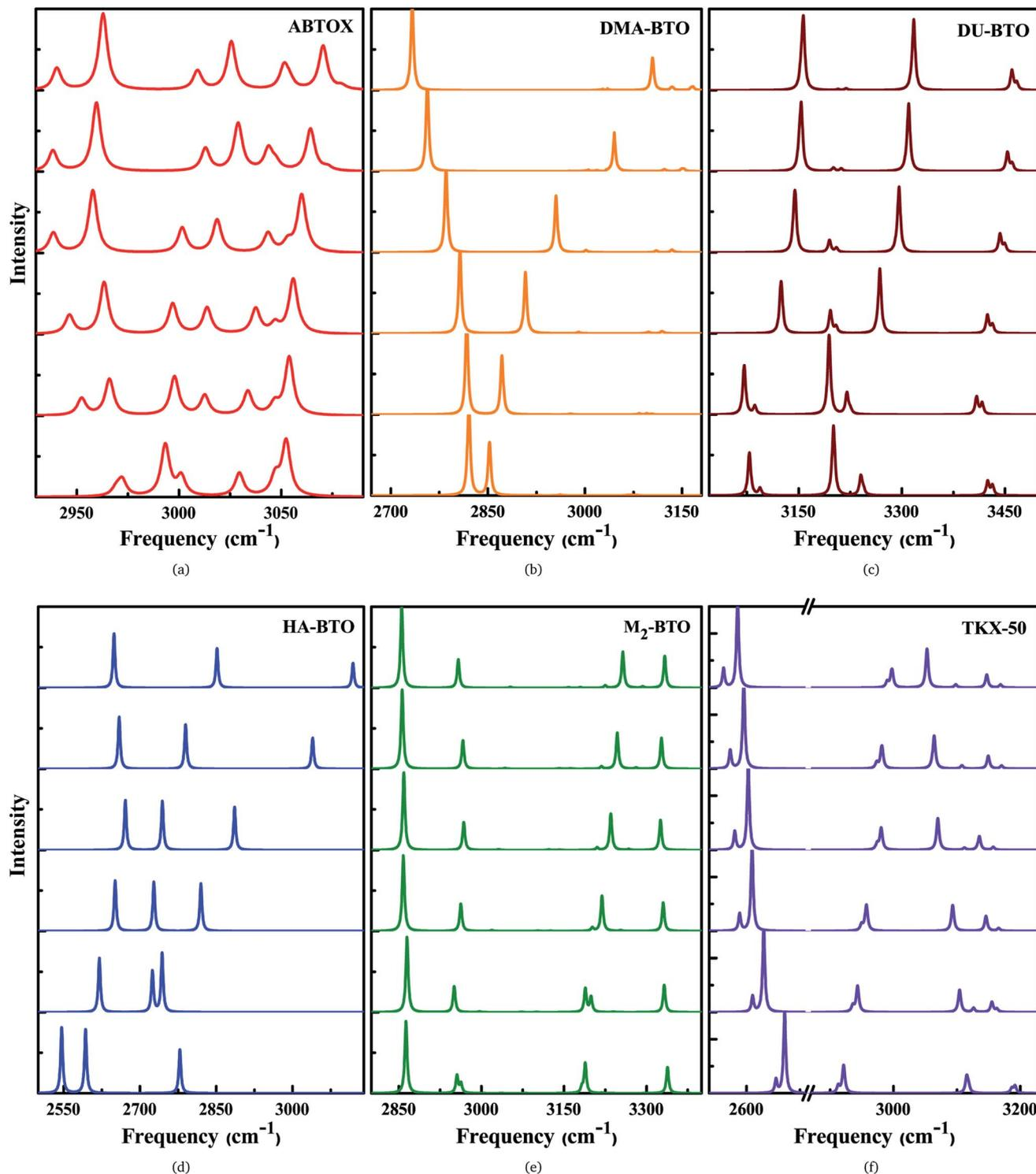
Fig. 5 Calculated pressure induced IR spectra of high frequency symmetric/asymmetric stretching vibrations for (a) ABTOX, (b) DMA-BTO, (c) DU-BTO, (d) HA-BTO, (e)  $M_2$ -BTO and (f) TKX-50 as a function of pressure up to 10 GPa.
