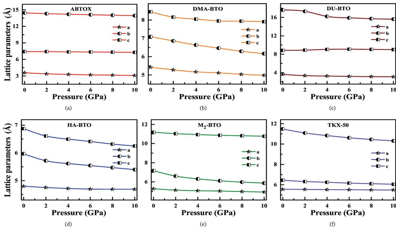
Fig. 3 Calculated unit cell parameters (*a*, *b*, *c*) for (a) ABTOX, (b) DMA-BTO, (c) DU-BTO, (d) HA-BTO, (e) M<sub>2</sub>-BTO and (f) TKX-50 as a function of pressure up to 10 GPa.
