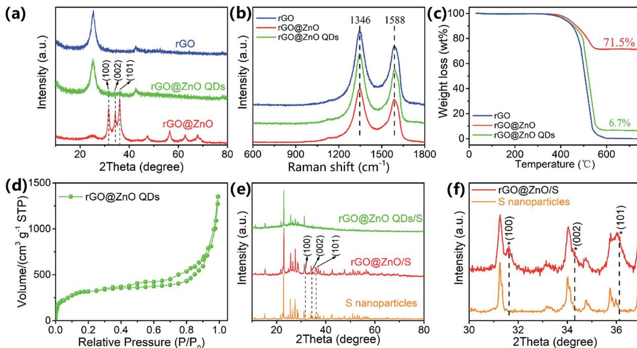
Fig. 3 (a) XRD patterns, (b) Raman spectra, and (c) TGA curves of rGO, rGO@ZnO, and rGO@ZnO QDs; (d) N<sub>2</sub> adsorption and desorption isotherm of rGO@ZnO QDs; (e) XRD patterns of S nanoparticles, rGO@ZnO/S and rGO@ZnO QDs/S; (f) partially enlarged XRD patterns of S nanoparticles and rGO@ZnO/S.
