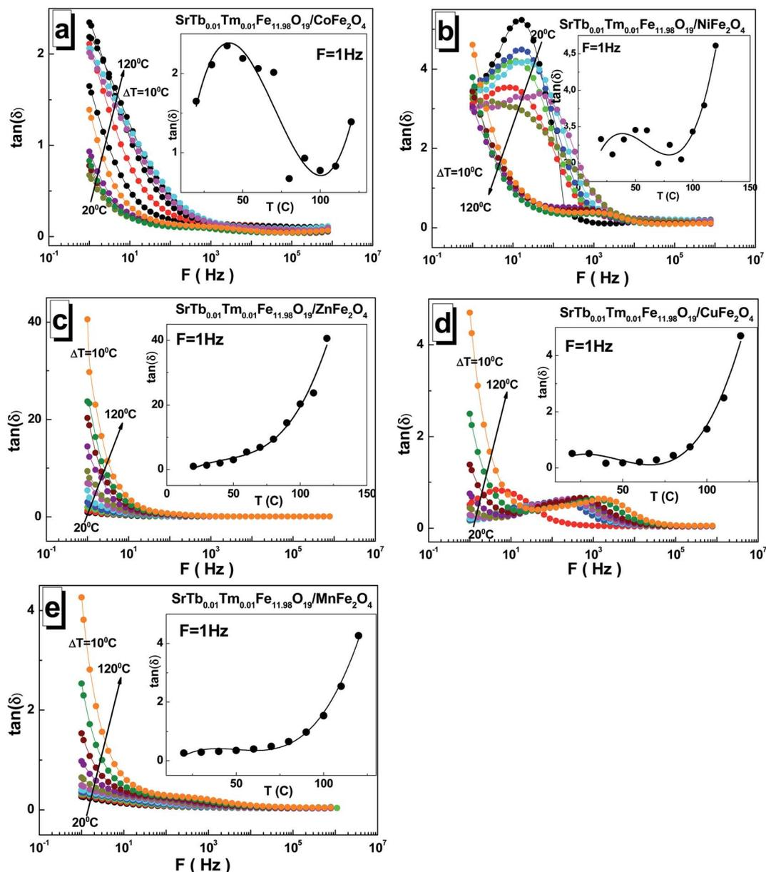
Fig. 6 Frequency dependences of the dielectric loss tangent  $\tan(\delta)$  in the range of  $1\text{--}3 \times 10^6$  Hz at different temperatures ranging from  $20^\circ\text{C}$  to  $120^\circ\text{C}$  with a step of  $\Delta T = 10^\circ\text{C}$  for the STTFO/AFer<sub>2</sub>O<sub>4</sub> functional composites, where A = Co (a), Ni (b), Zn (c), Cu (d), and Mn (e). Insets demonstrate the temperature dependence of  $\tan(\delta)$  at  $F = 1$  Hz.
