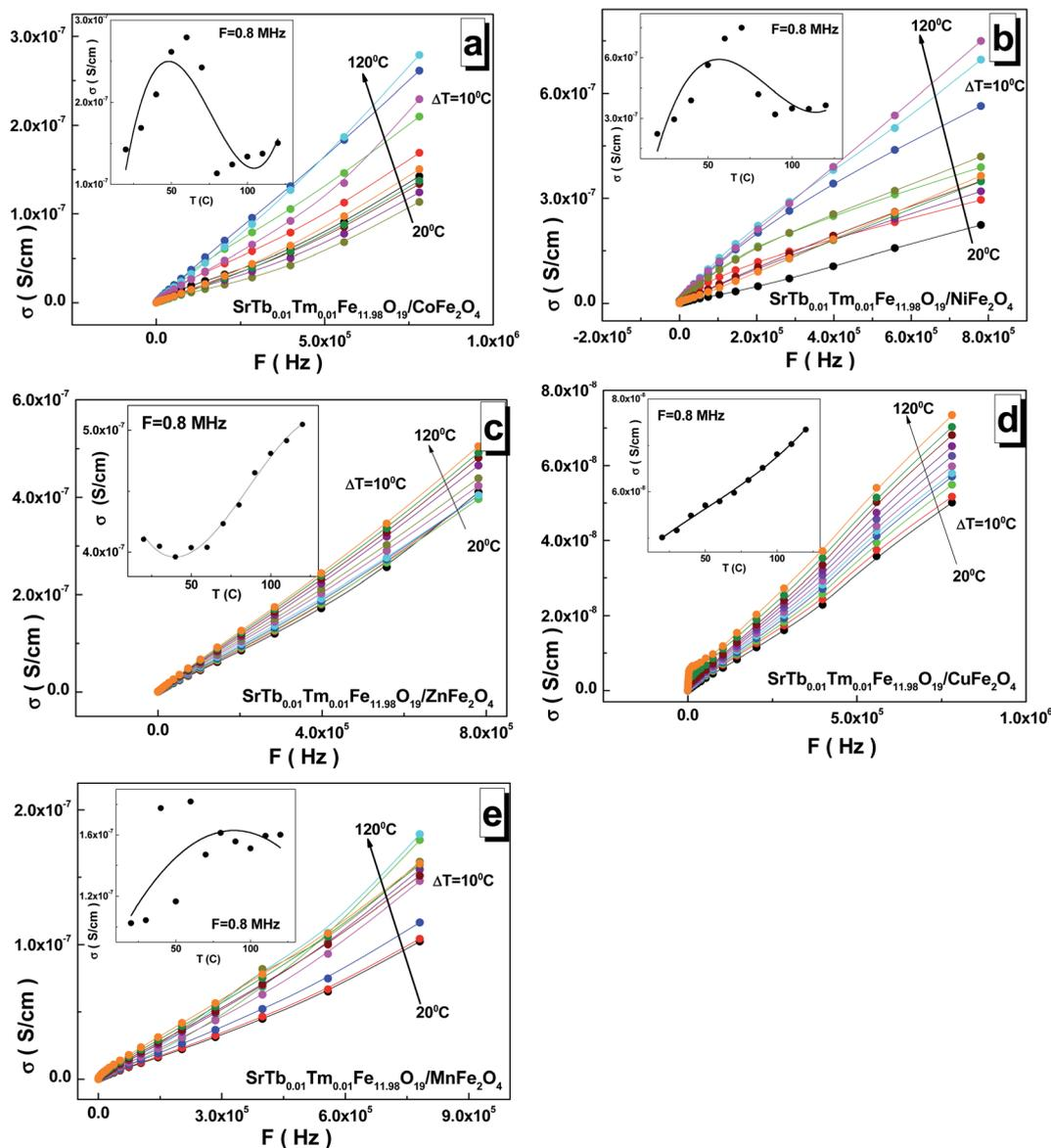
Fig. 7 Frequency dependences of the AC-conductivity in the range of  $1\text{--}3 \times 10^6$  Hz at different temperatures ranging from 20 °C to 120 °C with a step of  $\Delta T = 10$  °C for the STTFO/AF<sub>2</sub>O<sub>4</sub> functional composites, where A = Co (a), Ni (b), Zn (c), Cu (d), and Mn (e). Insets demonstrate the temperature dependence of the AC-conductivity at  $F = 0.8$  MHz.
