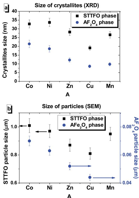
Fig. 3 The values of the average crystallite size (obtained using the XRD data) (a) and most probable particle size (obtained using the SEM images) for the (b) STTFO (black square) and AF<sub>2</sub>O<sub>4</sub> (blue circle) phases of each STTFO/AF<sub>2</sub>O<sub>4</sub> (A = Co, Ni, Zn, Cu, or Mn) functional composite.
