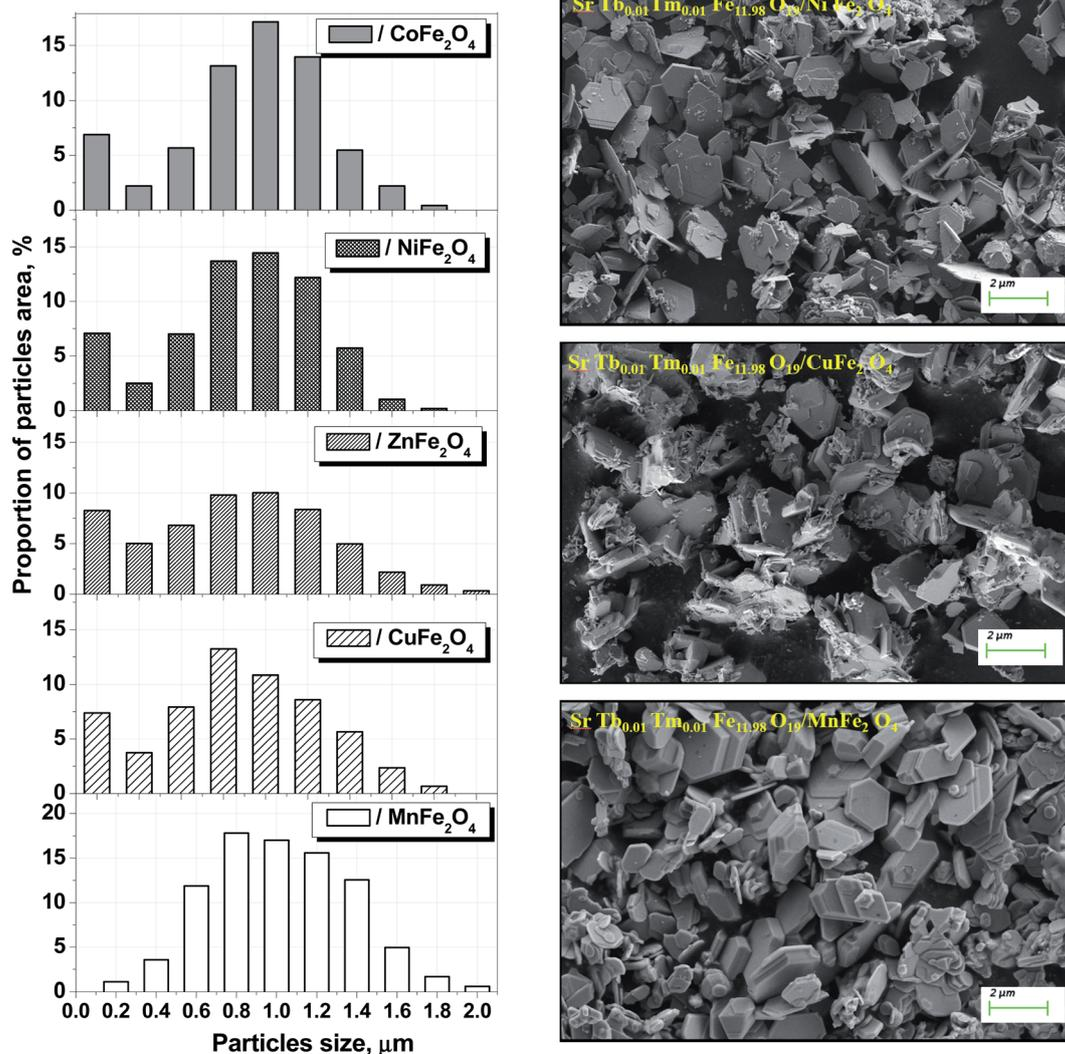
Fig. 2 Size distribution and SEM images of the composite particles for each STTFO/AFe<sub>2</sub>O<sub>4</sub> (A = Co, Ni, Zn, Cu, or Mn) functional composite.
