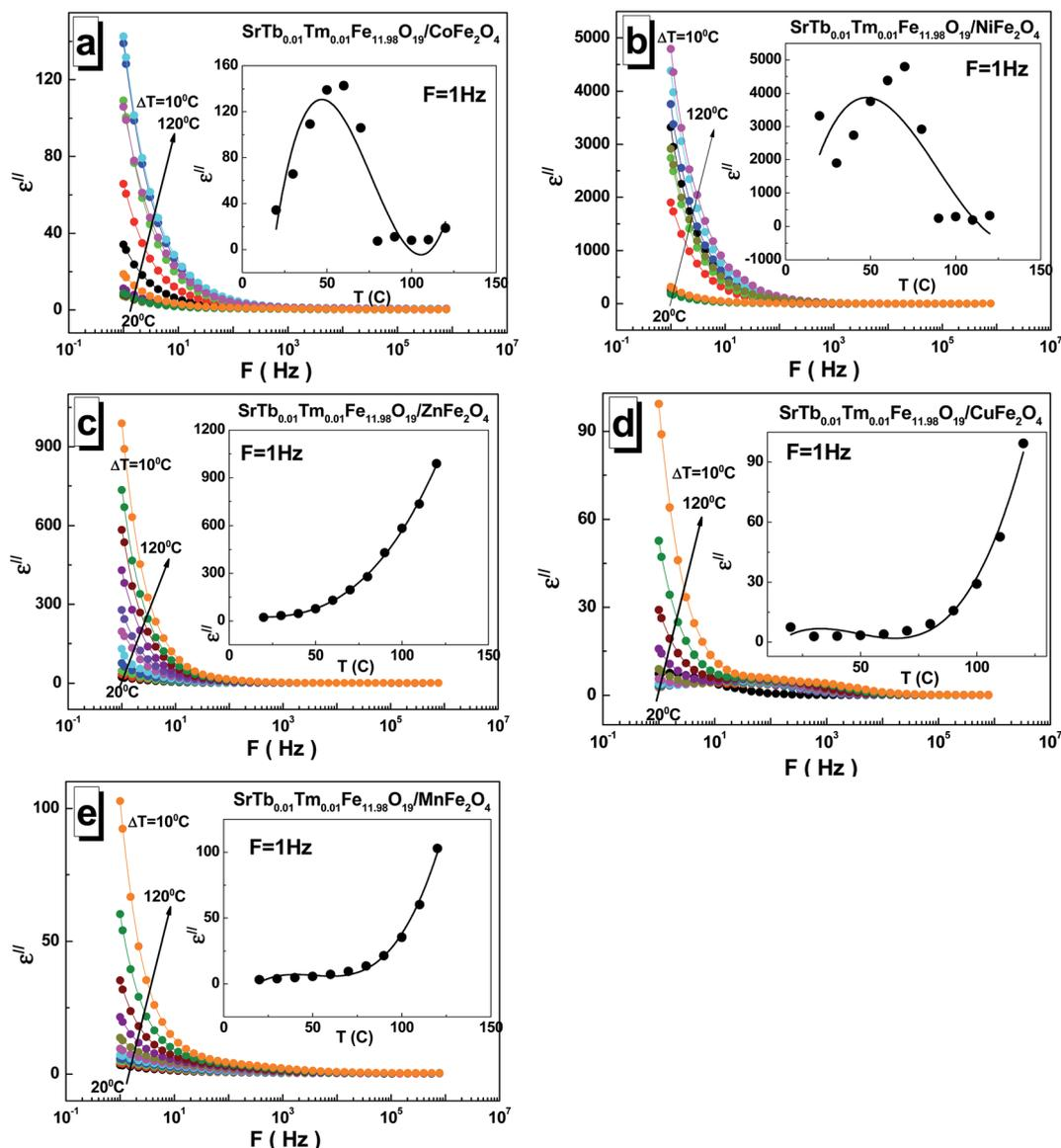
Fig. 5 Frequency dependences of the imaginary part  $\epsilon''$  of permittivity in the range of  $1\text{--}3 \times 10^6$  Hz at different temperatures ranging from  $20^\circ\text{C}$  to  $120^\circ\text{C}$  with a step of  $\Delta T = 10^\circ\text{C}$  for the STTFO/ $\text{AFFe}_2\text{O}_4$  functional composites, where A = Co (a), Ni (b), Zn (c), Cu (d), and Mn (e). Insets demonstrate the temperature dependence of the  $\epsilon''$  at  $F = 1$  Hz.
