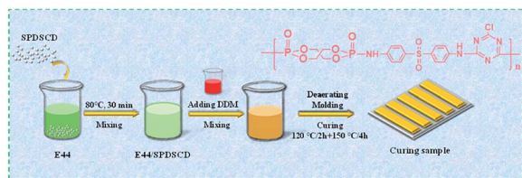
Fig. 1 The preparation process of SPDSCD/EP spline.
