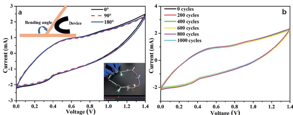
Fig. 6 (a) CV curves of the device at scan rate  $20\ mV\ s^{-1}$  after bending with different angel (inset: the photo of the device being bent at  $180^\circ$ ); (b) CV curves at  $20\ mV\ s^{-1}$  of the all-solid-state supercapacitor device being bent at  $180^\circ$  for different times.
