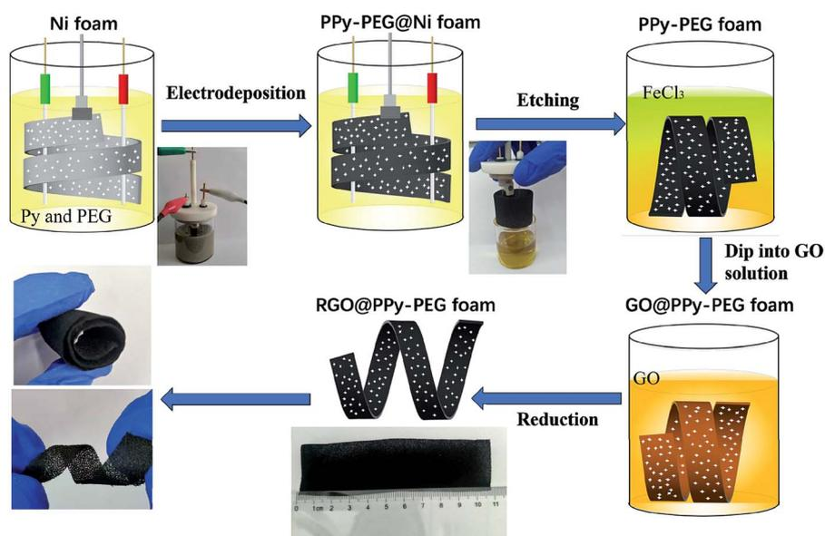
**Scheme 1** Schematic diagram and accompanying photographs of the fabrication of flexible, lightweight, and conductive RGO@PPy-PEG foams.
