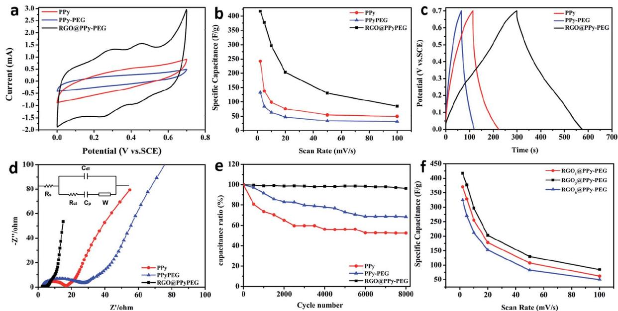
Fig. 4 (a) Comparison of CV curves at scan rate  $2 \text{ mV s}^{-1}$  and (b) plots of specific capacitance versus scan rate for PPy, PPy-PEG and RGO@PPy-PEG foam; (c) GCD curves at current density  $1 \text{ A g}^{-1}$  of PPy, PPy-PEG and RGO@PPy-PEG foam; (d) Nyquist plots and (e) cycling life of PPy, PPy-PEG, RGO@PPy-PEG foam; (f) plots of specific capacitance versus scan rate for RGO<sub>1</sub>@PPy-PEG, RGO<sub>3</sub>@PPy-PEG and RGO<sub>6</sub>@PPy-PEG.
