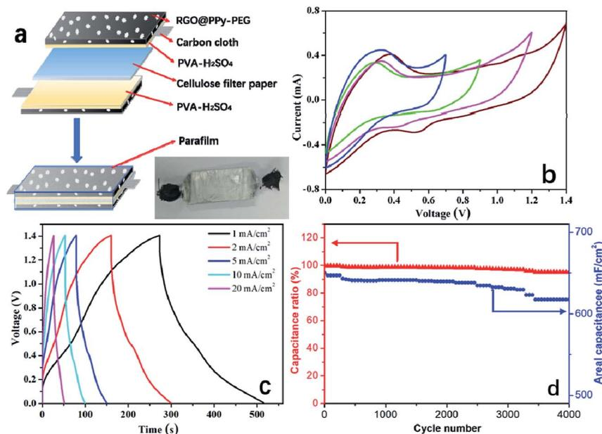
Fig. 5 (a) Illustration of the structure of the sandwich supercapacitors; (b) CV curves of the as-prepared symmetric supercapacitor at different voltage windows at a scan rate of  $2 \text{ mV s}^{-1}$ ; (c) GCD curves at various current densities; (d) cycling life of the device at a current density of  $10 \text{ mA cm}^{-2}$ .
