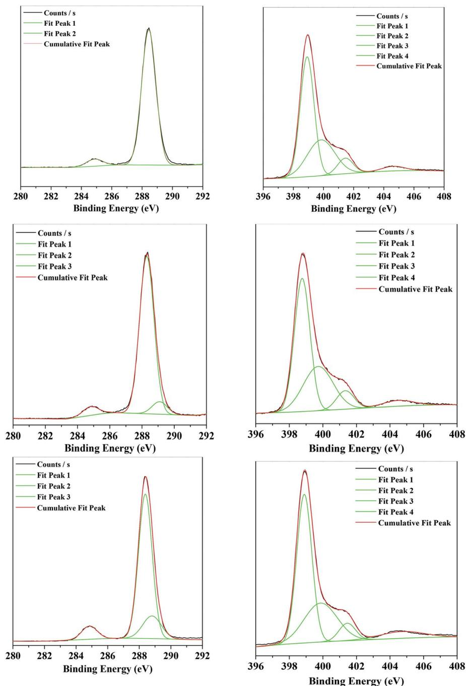
Fig. 4 XPS results of C1s (left) and N1s (right) for the various catalysts. (Top)  $g\text{-C}_3\text{N}_4$ , (middle)  $g\text{-C}_3\text{N}_4(\text{HY})$ , and (Bottom)  $g\text{-C}_3\text{N}_4(\text{HY-HT})$ .
