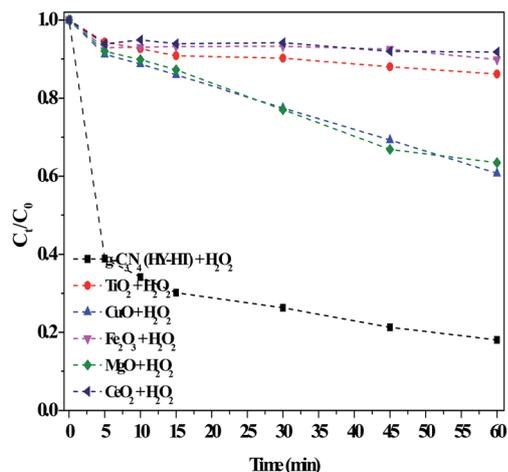
Fig. 5 Comparison of the performance of various heterogeneous catalysts for the degradation of RhB in the dark. Conditions:  $[\text{RhB}]_0 = 10 \text{ mg L}^{-1}$ ,  $[\text{H}_2\text{O}_2] = 36 \text{ mM}$ ,  $[\text{Catal.}] = 1.0 \text{ g L}^{-1}$ , initial pH no adjustment,  $25\text{ }^\circ\text{C}$  and 60 min.
