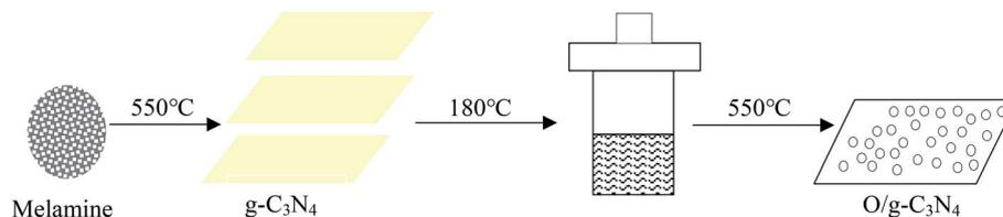
Scheme 1 Synthetic process to obtain O/g-C<sub>3</sub>N<sub>4</sub>.
