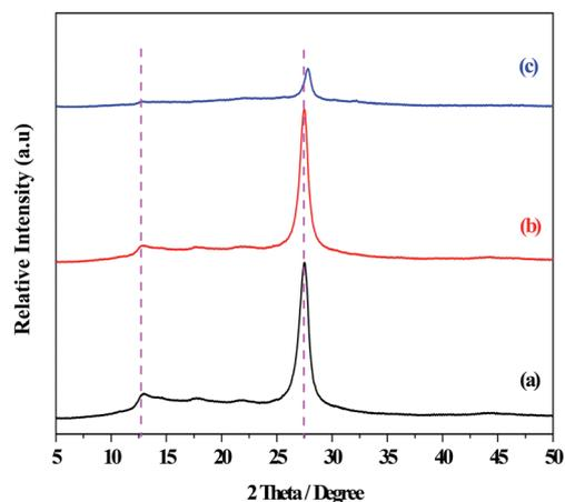
Fig. 1 XRD patterns of the series of catalysts. (a) g-C<sub>3</sub>N<sub>4</sub>, (b) g-C<sub>3</sub>N<sub>4</sub>(HY), and (c) g-C<sub>3</sub>N<sub>4</sub>(HY-HT).
