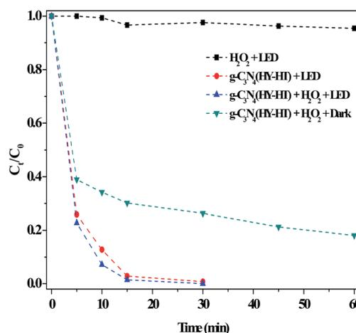
Fig. 7 Effect of the dark and light illumination on the degradation of RhB. Conditions:  $[\text{RhB}]_0 = 10 \text{ mg L}^{-1}$ ,  $[\text{H}_2\text{O}_2] = 36 \text{ mM}$ ,  $[\text{Catal.}] = 1.0 \text{ g L}^{-1}$ , initial pH no adjustment,  $25^\circ \text{C}$  and 60 min.
