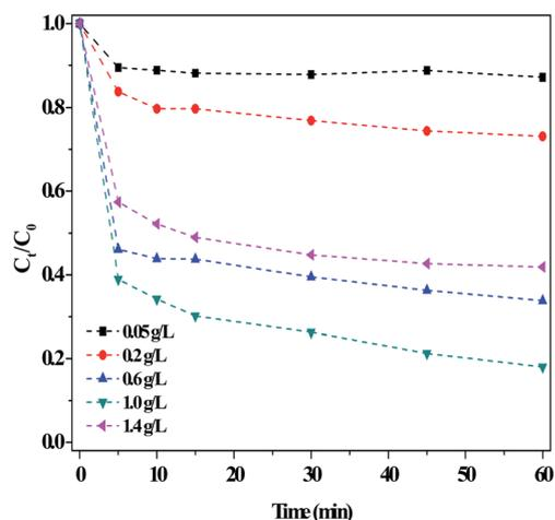
Fig. 8 Effect of the dosage of the g-C<sub>3</sub>N<sub>4</sub>(HY-HT) catalyst on the degradation of RhB in the dark. Conditions: [RhB]<sub>0</sub> = 10 mg L<sup>-1</sup>, [H<sub>2</sub>O<sub>2</sub>] = 36 mM, initial pH no adjustment, 25 °C and 60 min.
