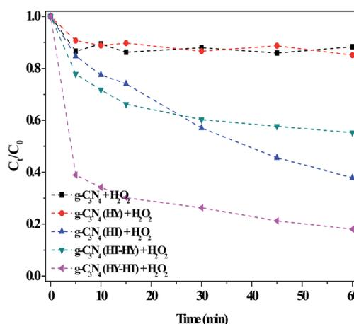
Fig. 6 Effect of the preparation method on the degradation of RhB in the dark. Conditions:  $[\text{RhB}]_0 = 10 \text{ mg L}^{-1}$ ,  $[\text{H}_2\text{O}_2] = 36 \text{ mM}$ ,  $[\text{Catal.}] = 1.0 \text{ g L}^{-1}$ , initial pH no adjustment,  $25\text{ }^\circ\text{C}$  and 60 min.
