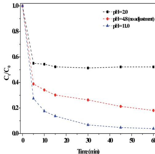
Fig. 9 Effect of adjusting the initial pH using H<sub>2</sub>SO<sub>4</sub> or NaOH on the degradation of RhB in the dark. Conditions: [RhB]<sub>0</sub> = 10 mg L<sup>-1</sup>, [Catal.] = 1.0 g L<sup>-1</sup>, [H<sub>2</sub>O<sub>2</sub>] = 36 mM, 25 °C and 60 min.
