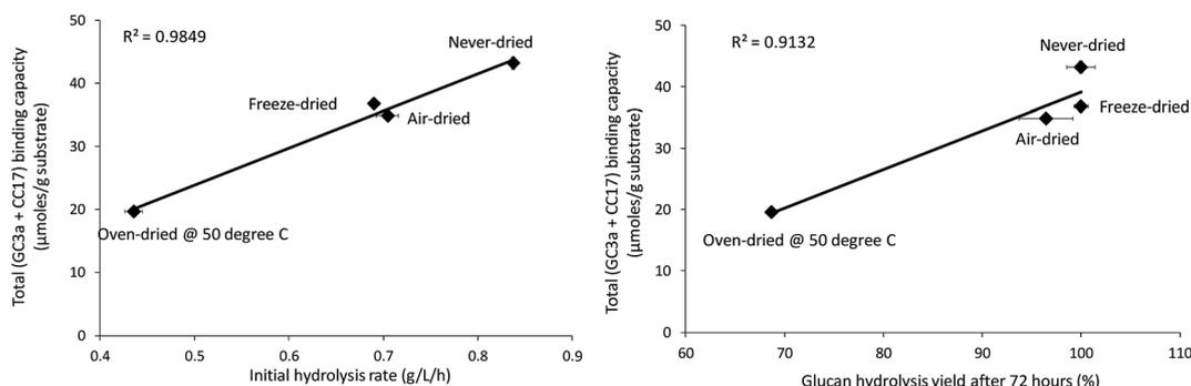
**Fig. 6** Correlation between total binding capacity, total cellulose accessibility (as determined by FP-CBM probes (GC3a + CC17)), and initial hydrolysis rates and cellulose hydrolysis yields (after 72 hours) of the dried and never-dried pulps.
