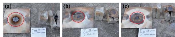
Fig. 6 The effects of thermite acting on the steel target plates under the restraint of stainless-steel tubes.
