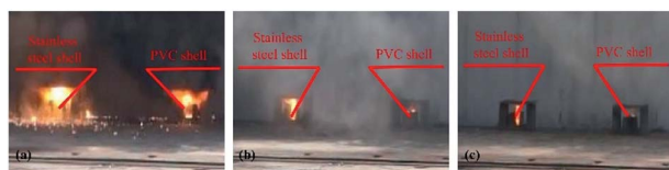
Fig. 5 Comparative experimental images of shells at different moments: (a) about 0.5 s, (b) about 1.5 s, and (c) about 2.5 s after ignition.
