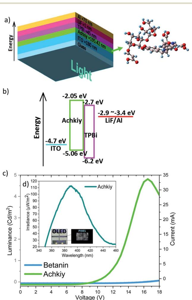
Fig. 9 (a) OLED sandwich structure and thicknesses of each thin layers. (b) The band gap energy (eV). (c) Voltage curve (V), current (mA) and luminance ( $\text{Cd m}^{-2}$ ) of the Achkiy and Betanin OLED. (d) Device irradiance curve.
