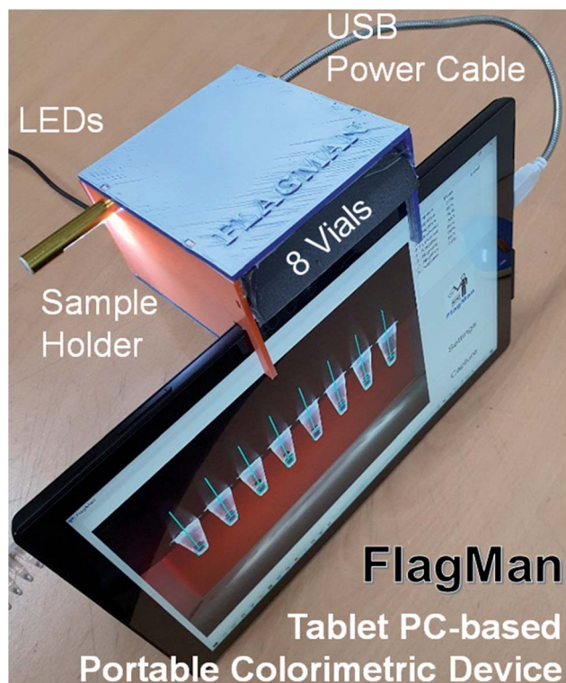
Fig. 7 Tablet PC-based portable colorimetric detection device with an enclosed sample holder designed for consistent lighting conditions.
