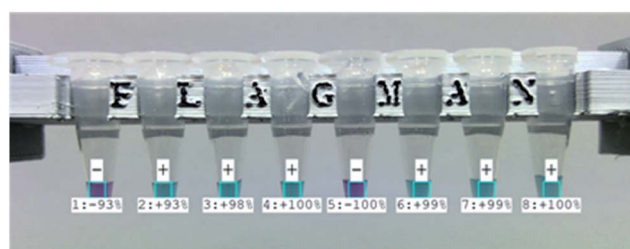
Fig. 5 Automatically captured and exported image of eight vials with test results and levels of confidence.
