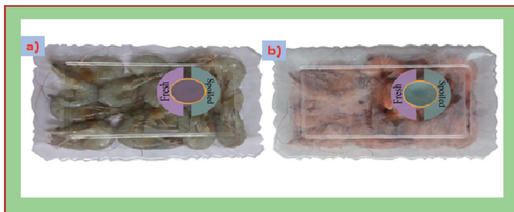
Fig. 7 Color changes in the intelligent pH indicator starch based films (S/BPE/TiO 2 ) attached to packages of prawn seafood sample (a) immediately after packaging (b) after 6 days of storage at 4 °C.
