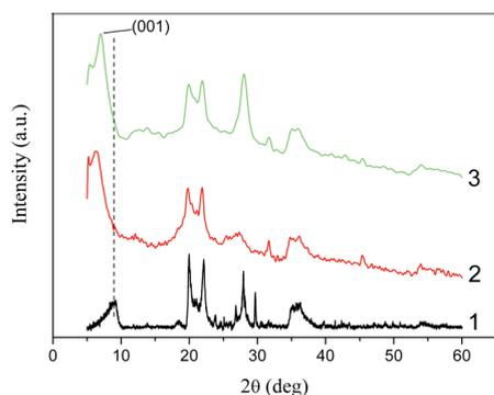
Fig. 8 WAXS patterns for Na-MMT (1), Na-MMT/BMImNTf<sub>2</sub> (2), and Na-MMT/EMImNTf<sub>2</sub> (3).
