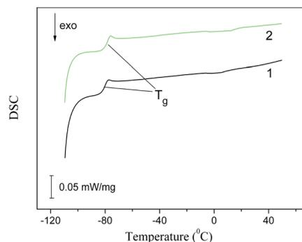
Fig. 10 DSC traces of the second heating cycle for the Bent/BMImNTf<sub>2</sub> (1) and Na-MMT/BMImNTf<sub>2</sub> (2) composites.
