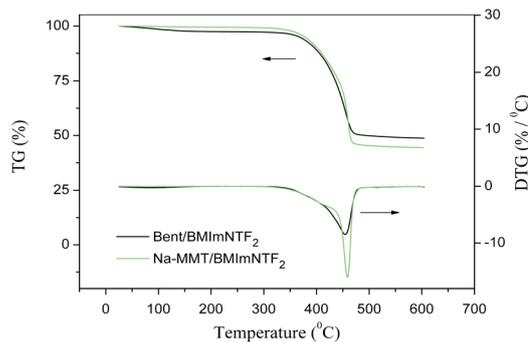
Fig. 12 TG and DTG traces recorded for the clay/BMImNTf<sub>2</sub> ionogels.
