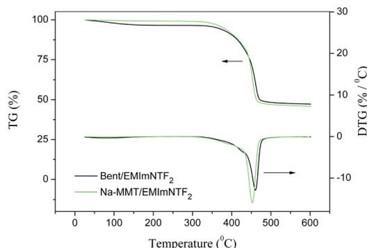
Fig. 13 TG and DTG traces recorded for the clay/EMImNTf<sub>2</sub> ionogels.
