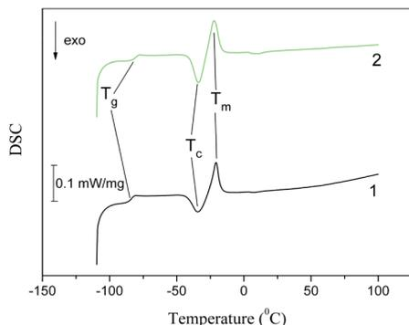
Fig. 11 DSC traces of the second heating cycle for the Bent/EMImNTf<sub>2</sub> (1) and Na-MMT/EMImNTf<sub>2</sub> (2) composites.
