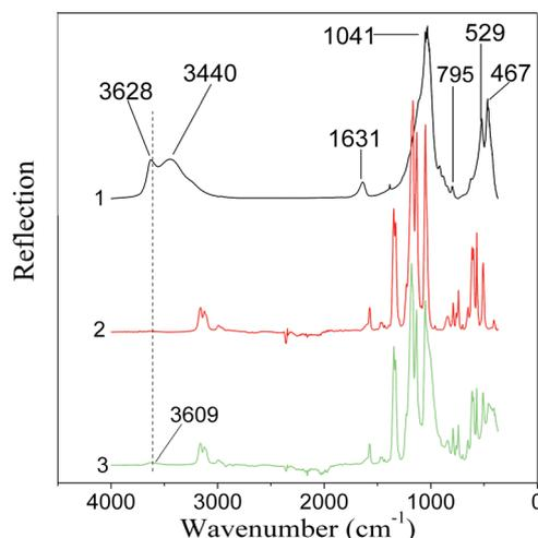
**Fig. 15** FTIR spectra of Na-MMT (1) EMImNTf<sub>2</sub> (2) and Na-MMT/EMImNTf<sub>2</sub> (3).
