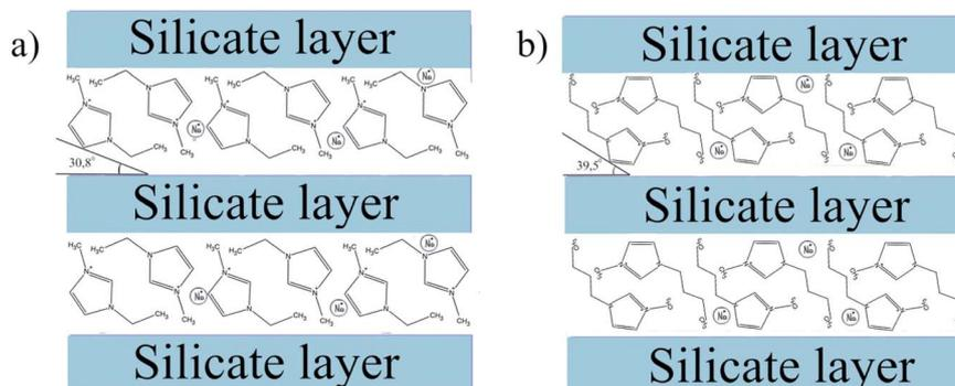
Fig. 9 Schematic structure of the Na-MMT/EMImNTf<sub>2</sub> (a) and Na-MMT/BMImNTf<sub>2</sub> ionogels.
