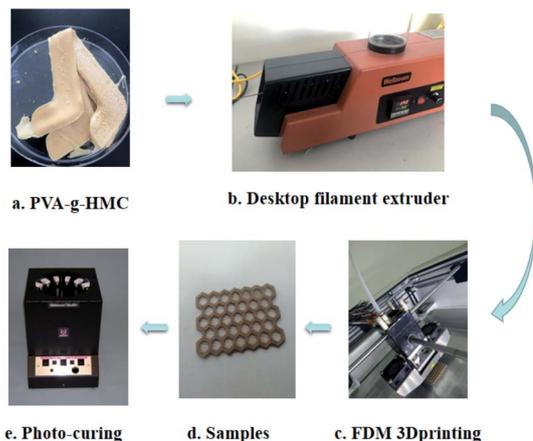
Fig. 9 Application of PVA-g-HMC in additive manufacturing.
