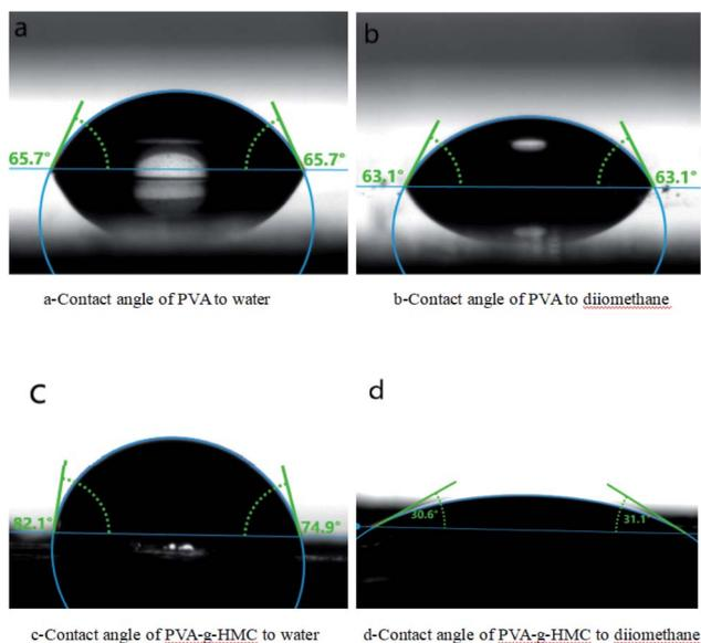
Fig. 8 Contact angle of PVA and PVA-g-HMC.
