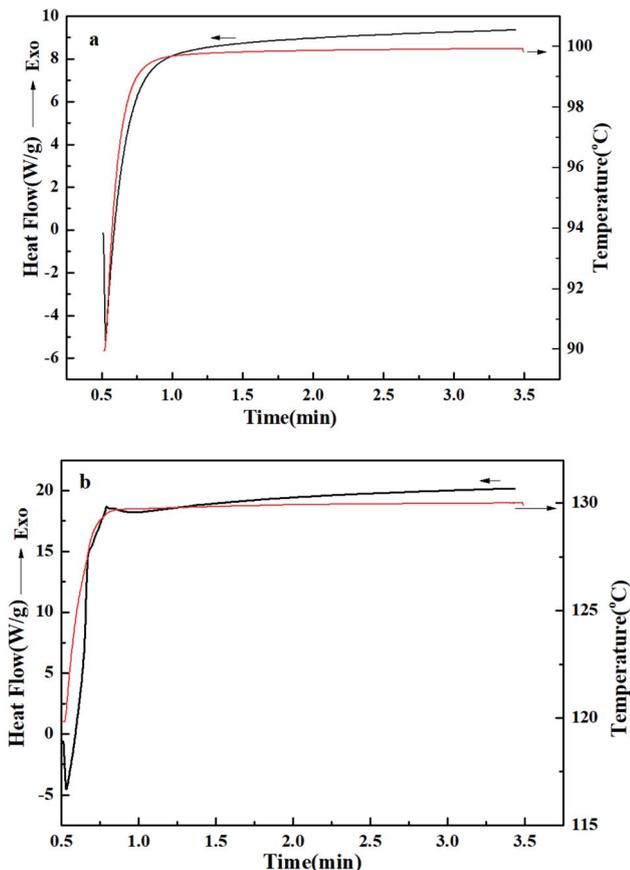
Fig. 6 UV-DSC curves of PVA-g-HMC at different temperatures: (a) at 130 °C, (b) at 140 °C.
