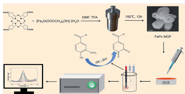
Scheme 1 Fabrication of FePc MOF/GCE modified electrode and electrochemical determination of vanillin.
